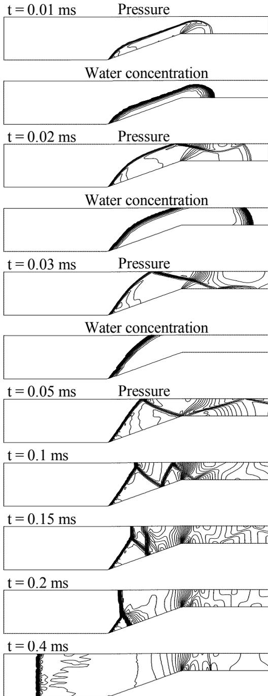
**Figure 7.** Detonation wave initiation and propagation by isobars and water concentration contours for case 1 ( $M_1=4.5$ ,  $\theta=20$  deg): only isobars for  $t \geq 0.05$  ms.
