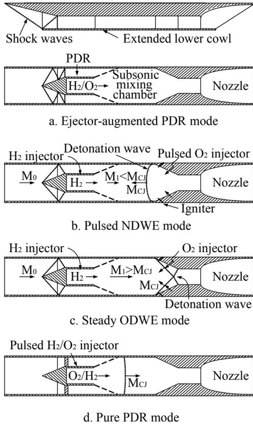
**Figure 1.** Schematic of multimode engine concept.<sup>1,2</sup>
