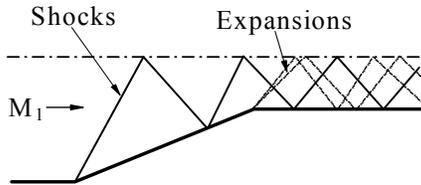
**Figure 3.** Induced shock and expansion waves by inert flow passing through the wedged channel.
