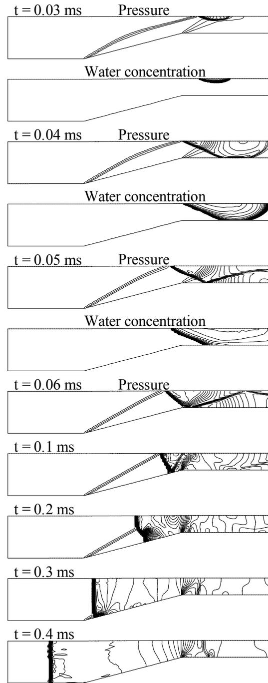
**Figure 8.** Detonation wave initiation and propagation by isobars and water concentration contours for case 2 ( $M_1=4$ ,  $\theta=15$  deg): only isobars for  $t \geq 0.06$  ms.
