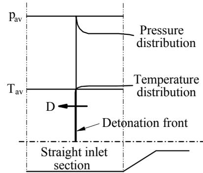
**Figure 15.** Schematic showing definitions of the average peak pressure and the corresponding average temperature and the detonation wave velocity.
