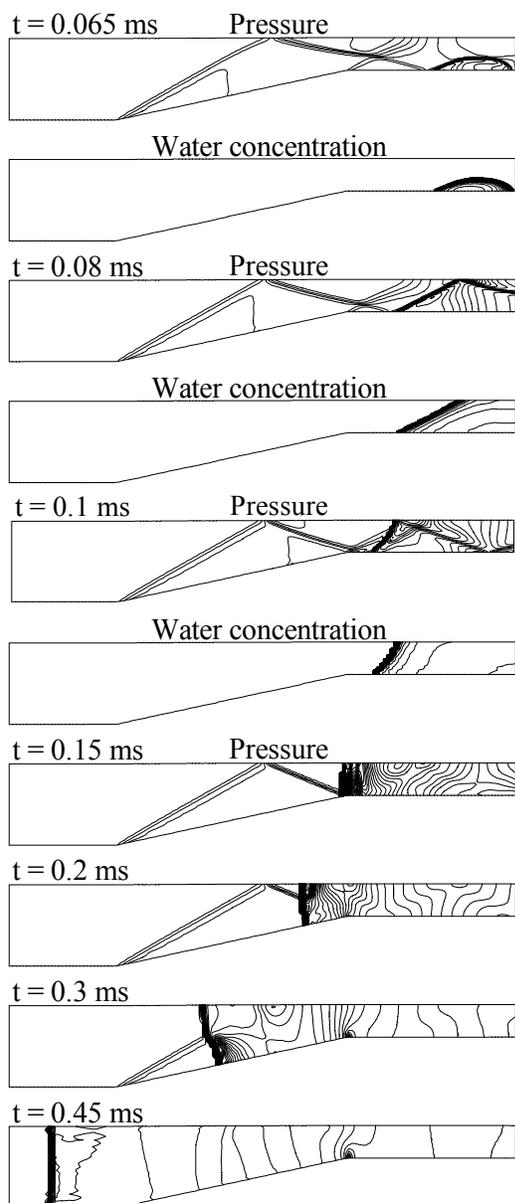
**Figure 9.** Detonation wave initiation and propagation by isobars and water concentration contours for case 3 ( $M_1=3.5$ ,  $\theta=12.5$  deg): only isobars for  $t \geq 0.15$  ms.
