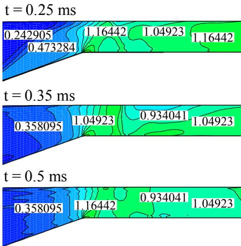
**Figure 14.** An indication of choking phenomenon in the outlet section of the channel (iso-Mach contours in laboratory frame).
