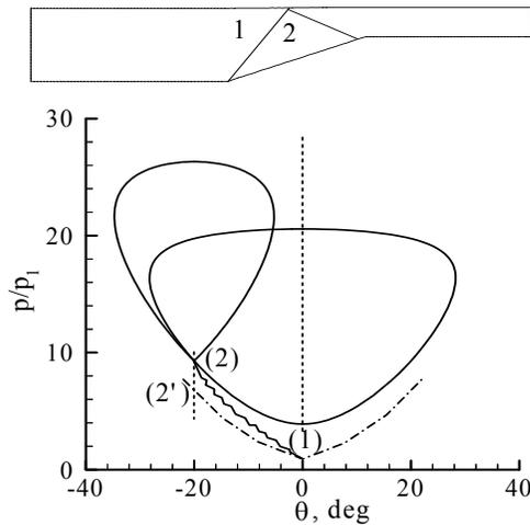
**Figure 11.** Polar diagram for the oblique detonation wave and its reflected shock for case 1.
