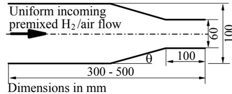
**Figure 2.** Schematic of the simplified wedged channel configuration.
