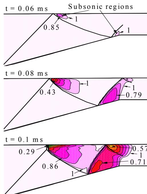
**Figure 10.** Subsonic flow regions produced in example case 1 (iso-Mach contours in laboratory frame).
