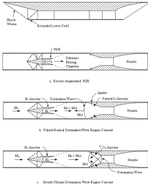
Figure 1: Schematic of proposed multimode engine
