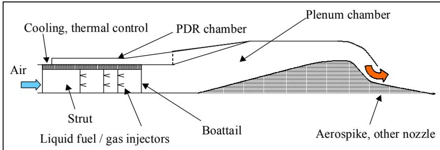
**Figure 4:** Top-mounted PDR with fuel injection struts
