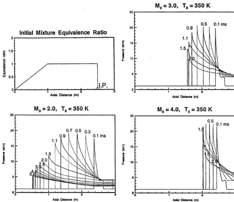
Figure 8: Detonation wave propagation into a mixing zone for Mode 2, T3 = 350 K
