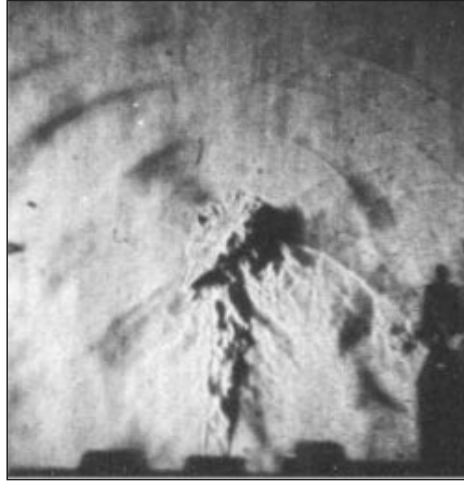
Figure 2 Supersonic flow (at the center of picture) disturbed by sonic generator (on the right side)
