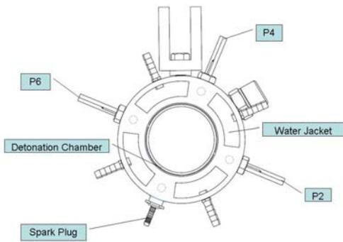
(a) First row of pressure transducers (P2, P4, P6) and spark plug.
