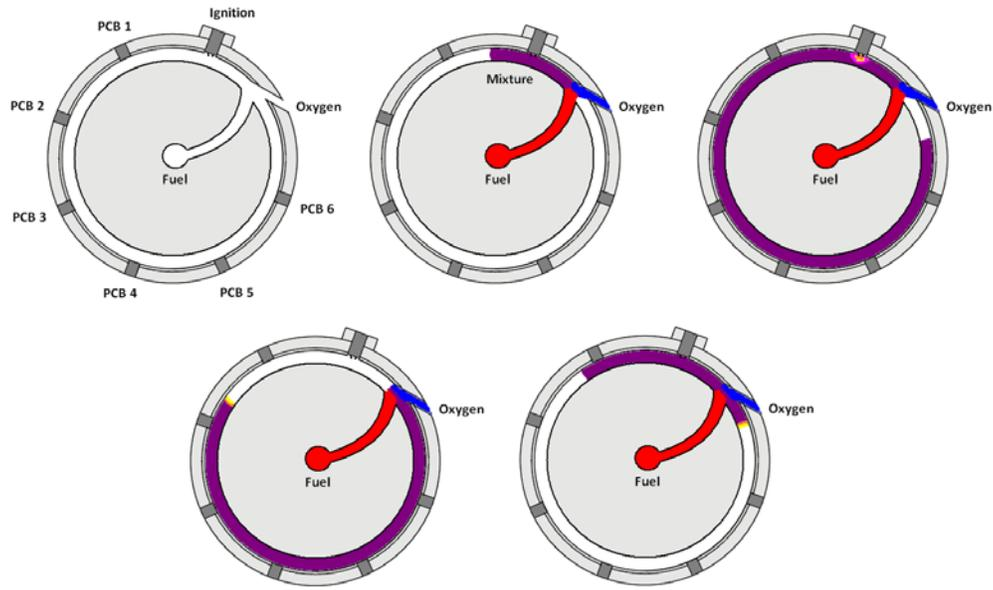
Figure 1. Schematic of the initiation cycle of the swirled-flow RDWE.
