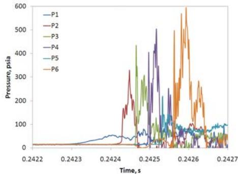
**Figure 8.** Pressure transducer readings from a hydrogen/oxygen test that shows the swirled fuel injection technique inducing a detonation wave in one direction around the annulus.
