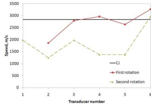
**Figure 9.** Wave diagram from a hydrogen/oxygen test showing an initial CJ detonation speed which degrades as the wave passes by the injector pair.
