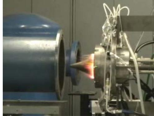
(b) Choked deflagration of fuel-rich propane/oxygen mixture.
