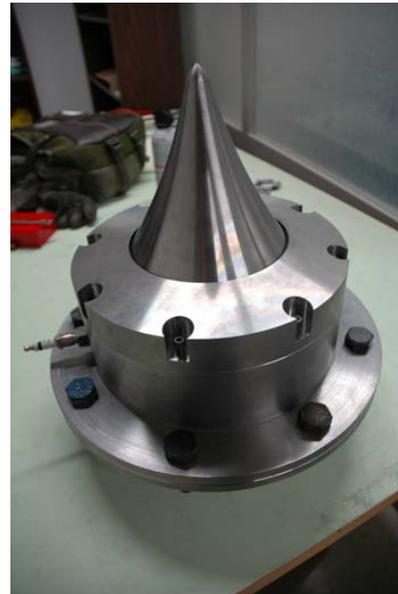
**Figure 3.** Photograph of the CDWE with the annular aerospace nozzle before mounting.
