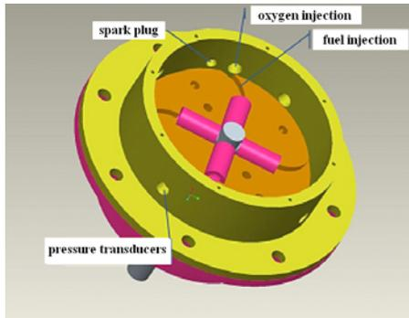
**Figure 2.** Computer-generated image of the CDWE annular chamber and central injection ports.
