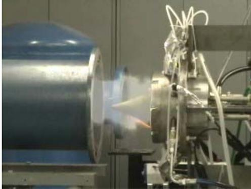
(a) Detonation of hydrogen/oxygen mixture.
