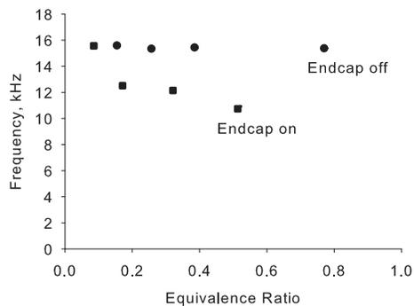
Figure 13. Frequency of detonation waves as a function of equivalence ratio.
