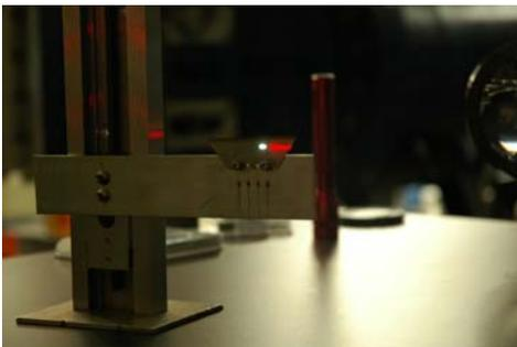
**Figure 4. Focal point (the bright point) at the knife edge revealing accuracy optical axis alignment with lasers.**
