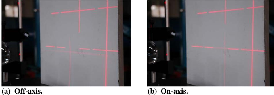
**Figure 1. Aligning optical components using a pair of aiming lasers with crosshair tips.**
