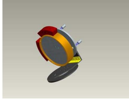
**Figure 2. Pro-Engineer Wildfire drawing of the customized mirror mounts.**
