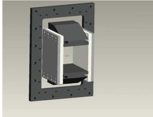
(b) Inlet nozzle with mounting bracket for assembly.
