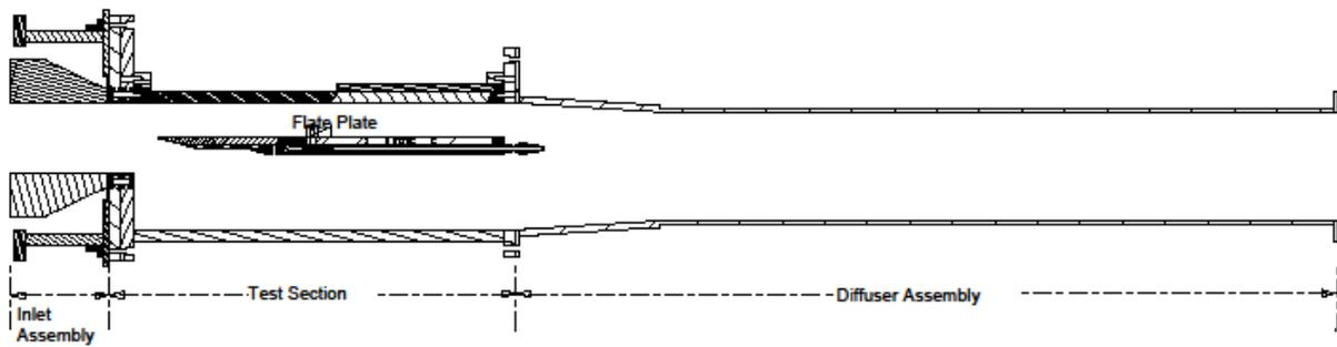
Figure 7. Full inlet, test section and diffuser assembly.
