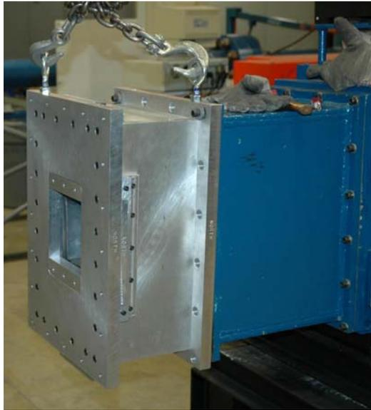
**Figure 4. Photograph of inlet adapter section on the blowdown supersonic tunnel.**
