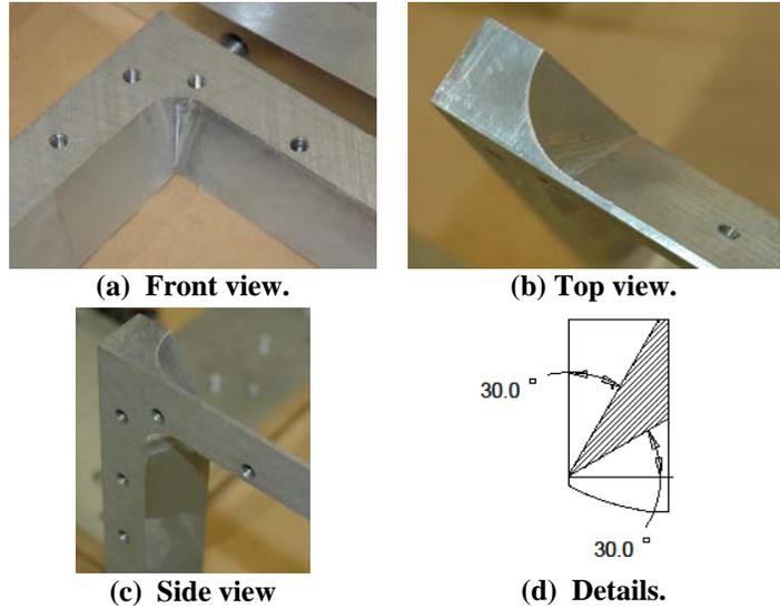
**Figure 5. Detailed photographs of the compound angle side walls.**
