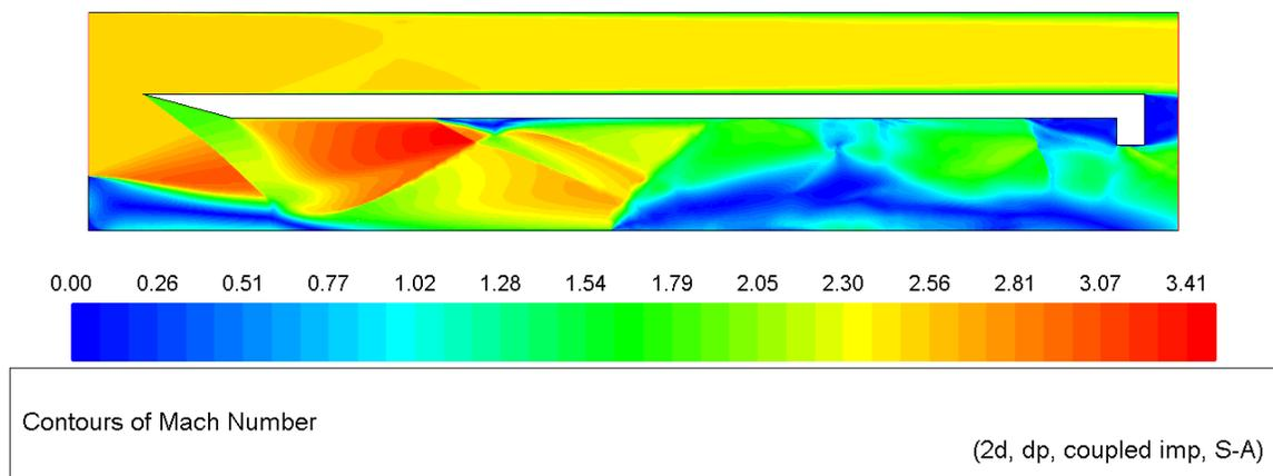
Figure 3. Mach number contours of initial flat plate design and test section dimensions ( $M = 2.5$ ).
