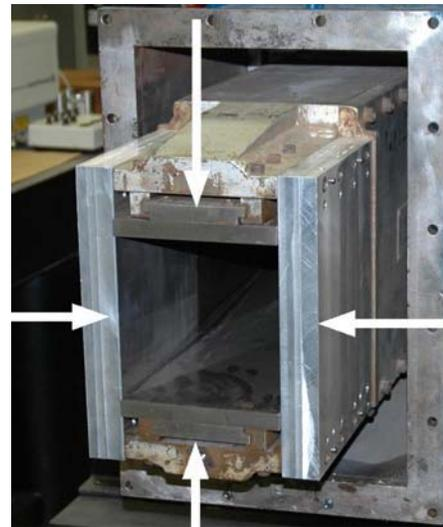
**Figure 2. Photograph of nozzle exit of the supersonic blowdown tunnel.**
