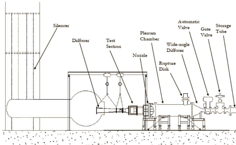
**Figure 1. Schematic of supersonic wind tunnel.<sup>15</sup>**
