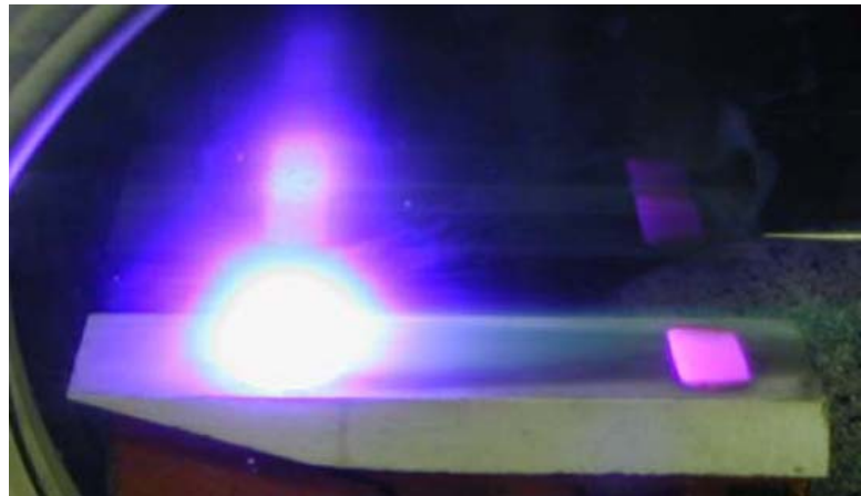
Figure 18. A DC voltage discharge between two electrodes at freestream conditions of M = 5.15 and p = 0.59 torr. The applied voltage is 880-920 V at a current of 50 mA. The addition of a magnetic field significantly affects the plasma and creates a virtual hypersonic leading edge strake (from Ref. 93).
