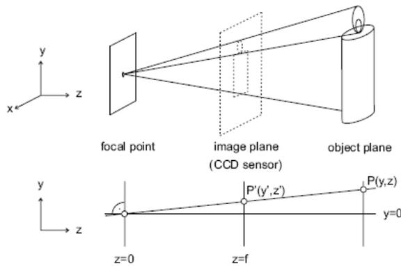
Fig. 6. Basic concept of the pinhole-fit model.<sup>17</sup>
