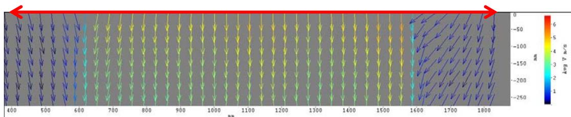
**Fig 9. Velocity vector profile of row 8 after the data from the four side-by-side rectangles were merged together. The solid red line represents the location (10 mm from the bottom of the air curtain exhaust) where the data of Fig. 10 were obtained.**
