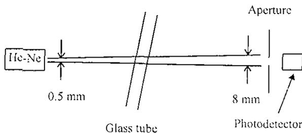
Fig. 2 Shock speed detection
