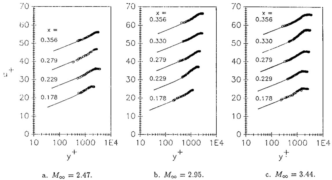
Figure 3: Undisturbed boundary-layer velocity profiles in wall coordinates.
