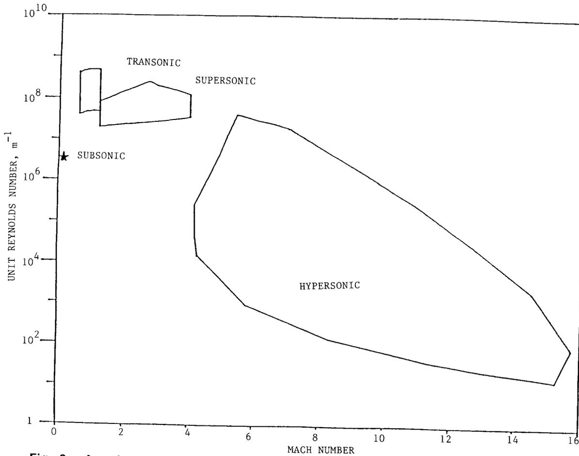
Fig. 2. Aerodynamics Research Center - Experimental Simulation Capability
