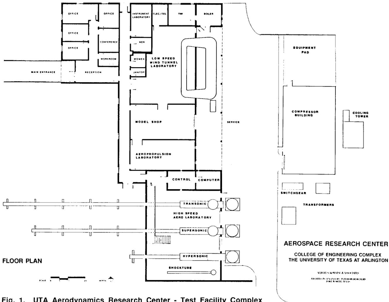
Fig. 1. UTA Aerodynamics Research Center - Test Facility Complex
