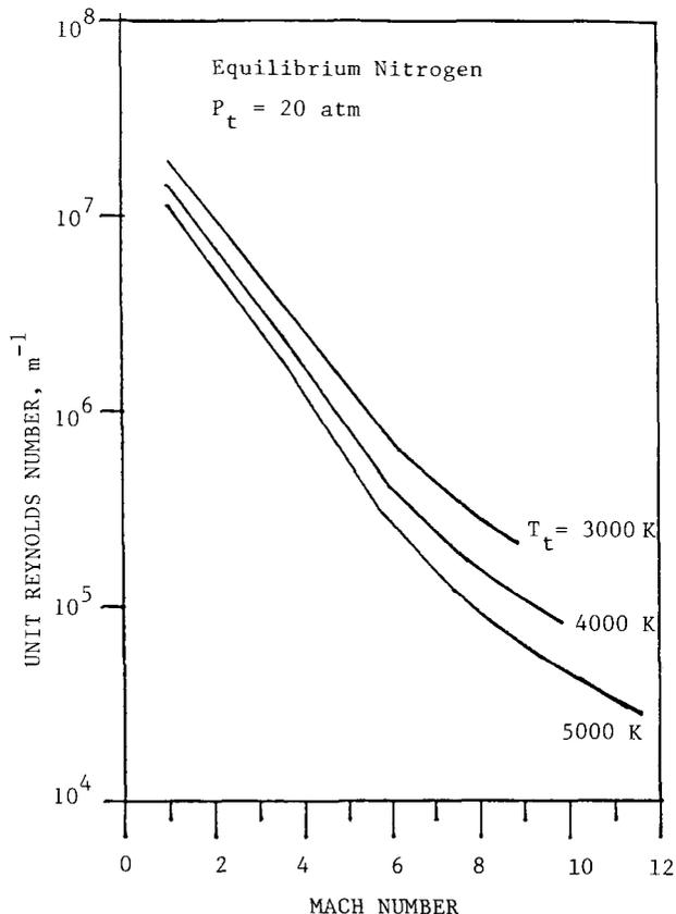
Fig. 10. Performance of Proposed Aerodynamic Heating Facility
