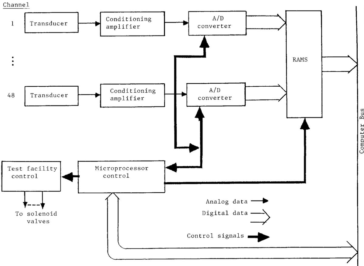
Fig. 11. Block Diagram-High Speed Data Acquisition/Control System
