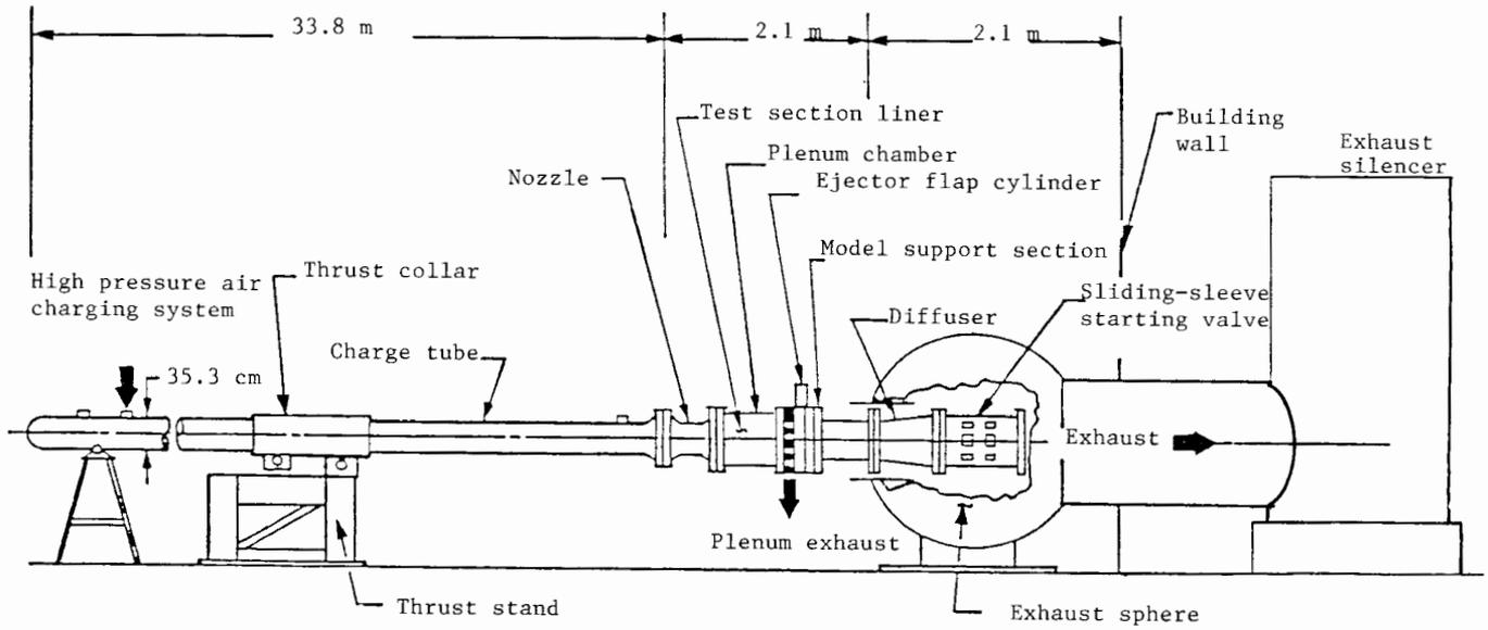
Fig. 4. Elevation View - Transonic Ludwieg Tube Wind Tunnel
