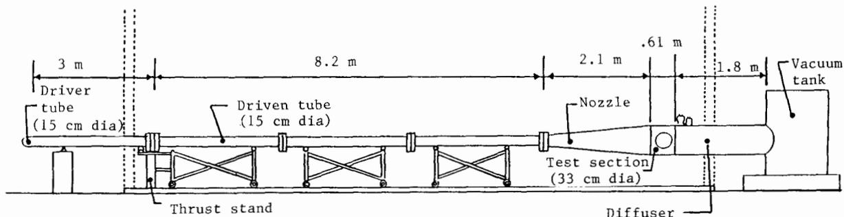
Fig. 7. Elevation View of Hypersonic Shock Tunnel
