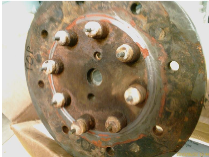
Figure 4. Corona electrodes mounted in head cap.
