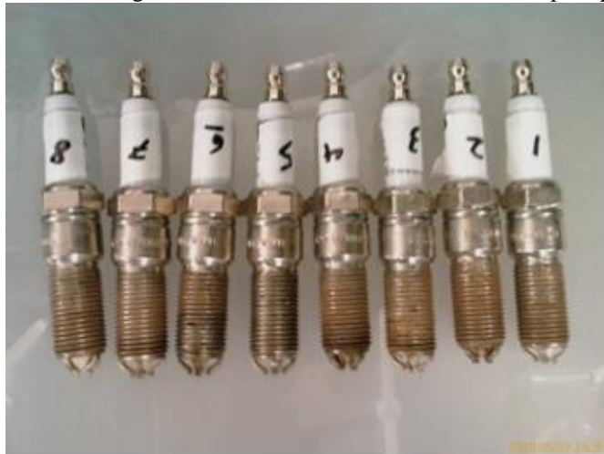
Figure 5. Spark plugs showing negligible degradation.
