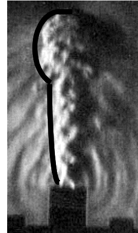
Figure 6. Whistler nozzle performance. Black line is contact surface contour that was used to calculate the symmetrical cross-sectional area of the jet plume.
