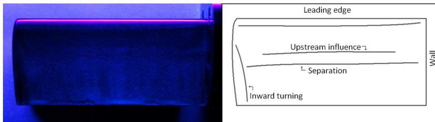
**Fig. 6** Fluorescent surface oil flow visualization of the airfoil at a 6 deg AOA, Mach 0.87, and  $Re = 3.27 \times 10^6$ .
