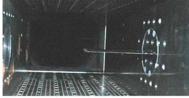
**Fig. 2** Test section showing the semispan wing with a NACA 0012 profile.
