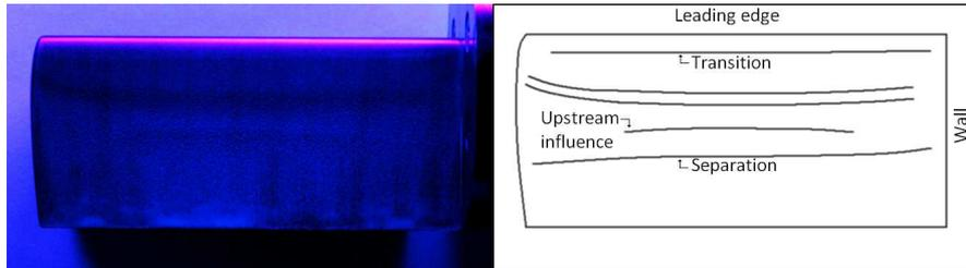
**Fig. 5** Fluorescent surface oil flow visualization of wing at zero incidence, Mach  $0.85 \pm 0.015$ , and  $Re = 3.24 \times 10^6$ .
