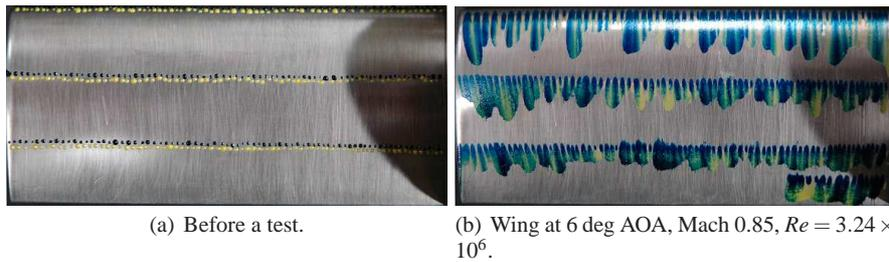
**Fig. 4** SFV results with oil flow dots.
