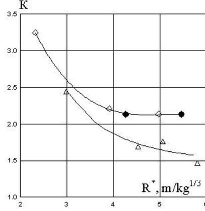
**Fig. 3.** The attenuation parameters:  $R^*$  - trajectory of sand front (triangles),  $K$  - attenuation coefficient (diamonds - 13 cm wall, circles - 8 cm wall, triangles - 5 cm wall)
