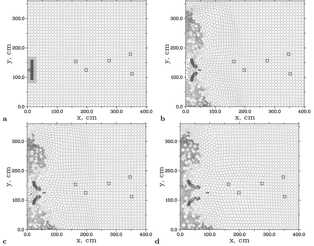
**Fig. 5.** Flow fields for 'confined' TNT explosion. Time moments 0.0, 2.6, 3.5 and 6.5 ms correspondingly. The pressure transducers positions are marked by squares. The material is presented by black circles for the sand/cement cylinder, by dark-grey circles for detonation products and light-grey circles for air. Left border is symmetry axis, other borders are chamber walls.
