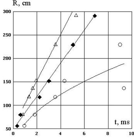
**Fig. 2.** The trajectory of blast wave for explosion without attenuator (triangles), the distance to epicenter normalized by equivalent TNT charge (diamonds) and trajectory of sand front (circles)
