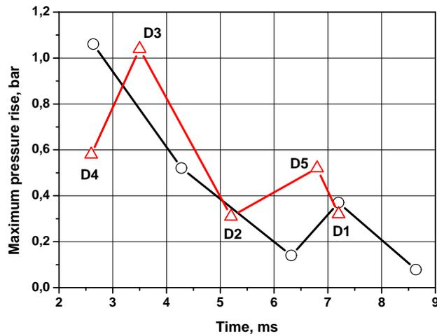
**Fig. 6.** Maximum pressure rise for TNT explosion in sand/cement cylinder at static pressure gauges  $D1$ ,  $D2$  and total pressure gauges  $D3$ – $D5$ . Measured values ( $\circ$ ) and computed values ( $\triangle$ ).
