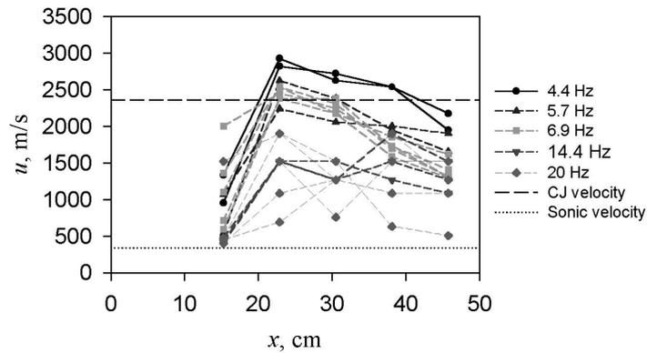
**Fig. 7.** Wave propagation for Shchelkin spiral configuration at various frequencies
