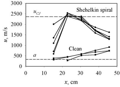
**Fig. 5.** Wave velocity at 6.9 Hz cycle frequency for clean and Shchelkin spiral configuration
