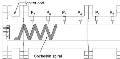
**Fig. 1.** Detonation chamber configuration: internal and external diameters of 7.62 and 15.2 cm respectively, length = 7.62, 15.2 or 30.5 cm; igniter located 3.81 cm from end wall, transducer P<sub>7</sub> located 7.62 cm from igniter and transducers thereafter are spaced at 7.62 cm intervals, P<sub>1</sub> (not shown) measures atmospheric pressure
