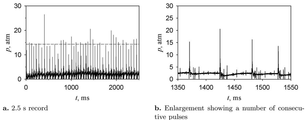
**Fig. 3.** Pressure record of transducer 6
