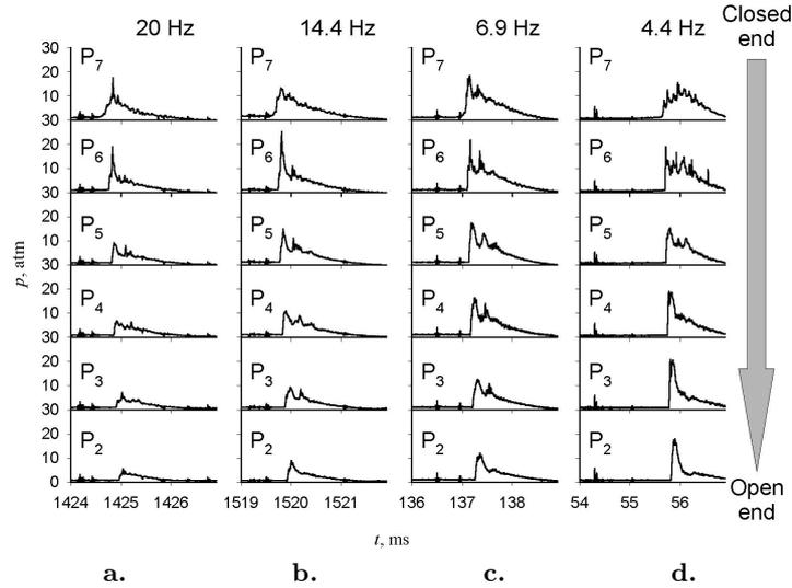
**Fig. 6.** Single pulse propagation comparison at various frequencies for the Shchelkin spiral configuration
