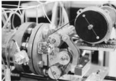
**Fig. 2.** Rotary valve assembly
