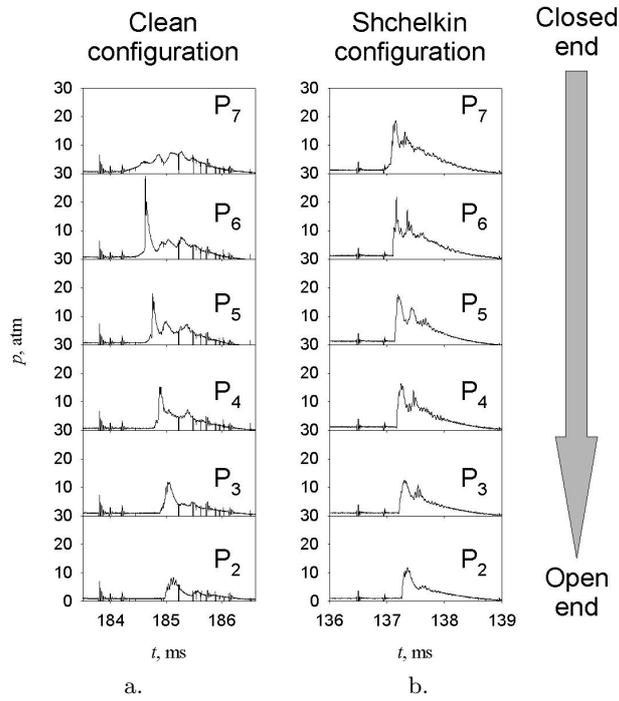
**Fig. 4.** Pressure profiles at 6.9 Hz cycle frequency
