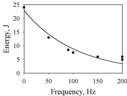
**Fig. 3.** Arc discharge measurements
