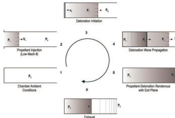
**Fig. 1.** Schematic of pulse detonation engine cycle
