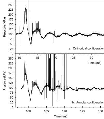
**Fig. 10.** Pressure traces near nozzle exit (single-shot experiment with stoichiometric oxygen-propane mixture at 1 atm initial conditions without Shchelkin spiral)
