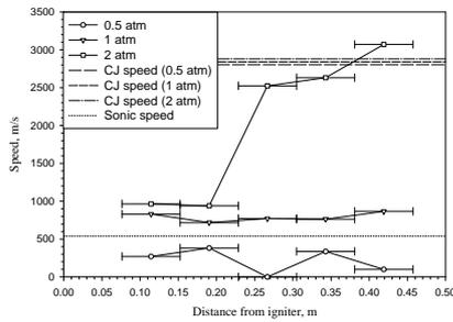
**Fig. 5.** Wave velocities for a stoichiometric  $H_2/O_2$  mixture at different initial pressures.
