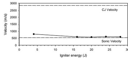
**Fig. 6.** Wave speed for different ignition energies for a stoichiometric  $H_2/O_2$  mixture at 1 atm (single-shot experiment).
