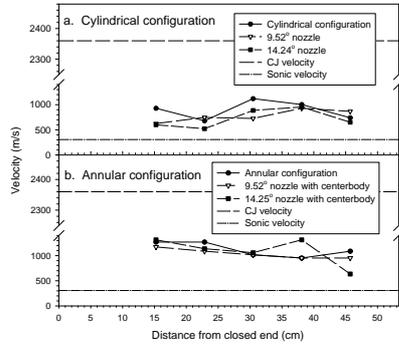
**Fig. 9.** Effect of nozzle on detonation wave propagation in a stoichiometric propane-oxygen mixture at 1 atm initial pressure (single-shot without Shchelkin spiral)
