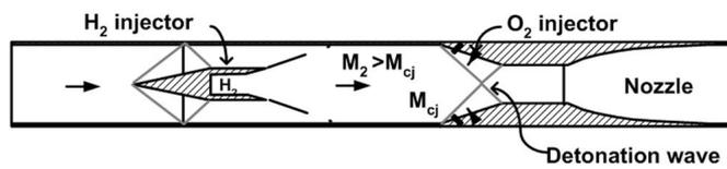
c. Steady oblique detonation wave engine
