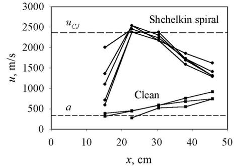
**Fig. 8.** Wave velocity at 6.9 Hz cycle frequency for clean and Shchelkin spiral configuration (stoichiometric oxygen-propane mixture at 1 atm initial conditions)
