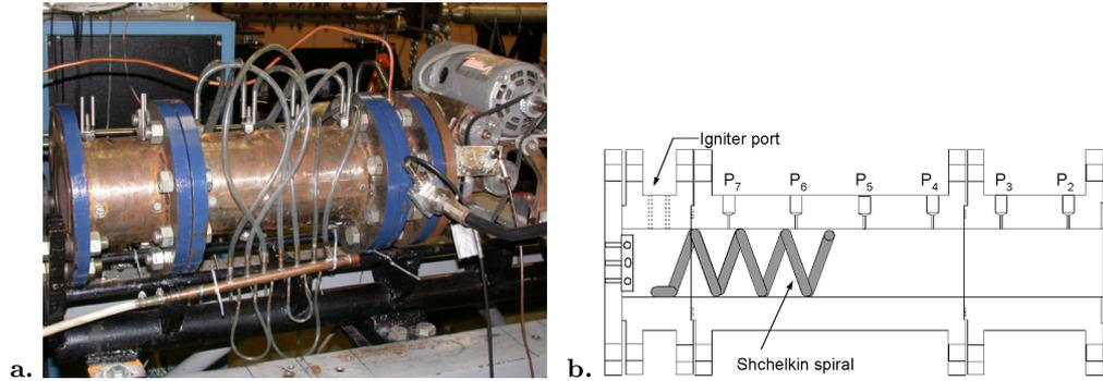
**Fig. 2.** Pulse detonation test rig. **a.** Photograph, flow from right to left; **b.** Schematic of detonation chamber with Shchelkin spiral
