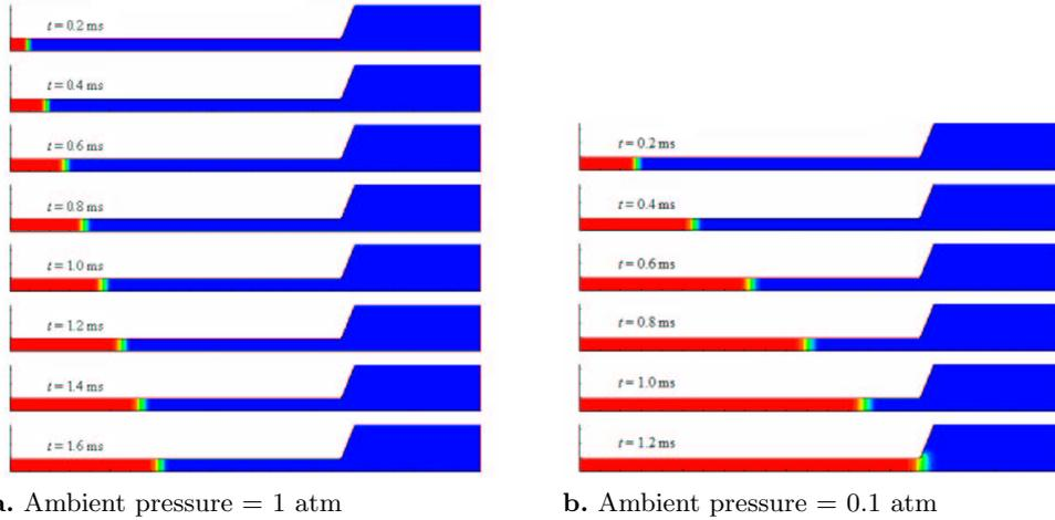
**Fig. 11.** Hydrogen concentration plots of wave propagation in a straight tube filled initially with a stoichiometric oxyhydrogen mixture at standard conditions
