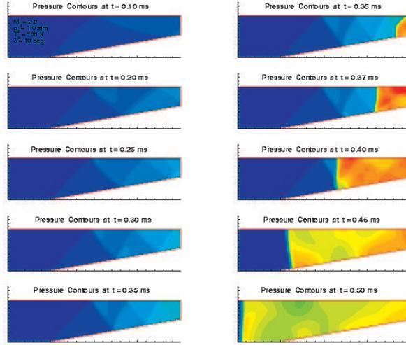
**Fig. 14.** Pressure contours showing shock initiation of unsteady detonation at low supersonic Mach numbers (flow from left to right)
