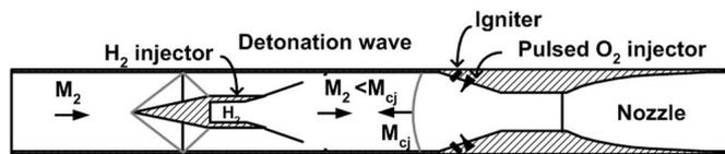
b. Pulsed normal detonation wave engine
