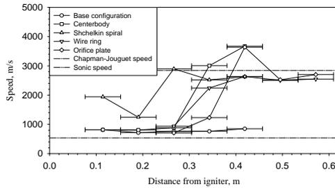
**Fig. 7.** Effect of enhancement devices on wave velocity for stoichiometric  $H_2/O_2$  mixtures at an initial pressure of one atm (single-shot experiment)
