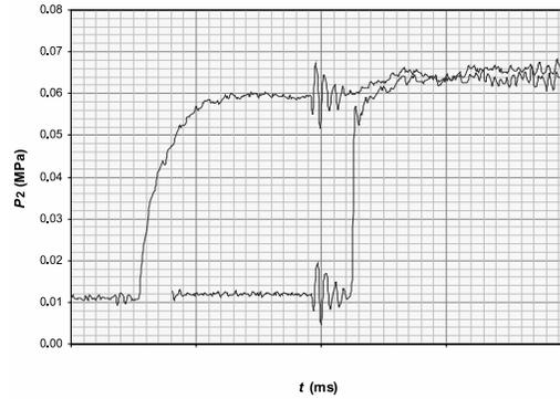
**Fig. 4.** Pressure profile from pressure transducers along the driven tube.
