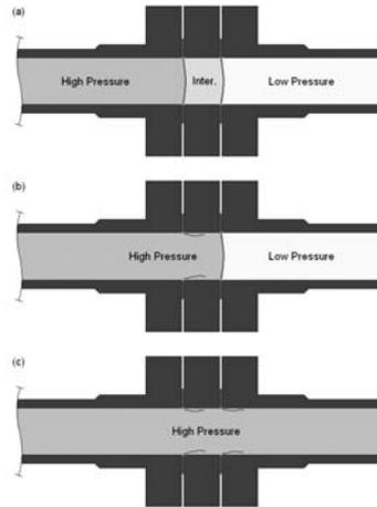
**Fig. 3.** The diaphragm rupture process. It begins with three initially separate regions (a). Pressure in the intermediate section is decreased to increase the pressure difference across the driver diaphragm (b). The ensuing rupture causes an equal pressure difference across the intermediate diaphragm (c).
