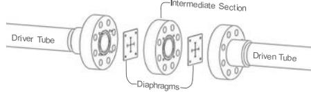
**Fig. 2.** Exploded view of diaphragm section shows the driver section diaphragm (left) and intermediate section diaphragm (right). Upon diaphragm rupture, air flows from the high pressure section (left) to the low pressure section (right).
