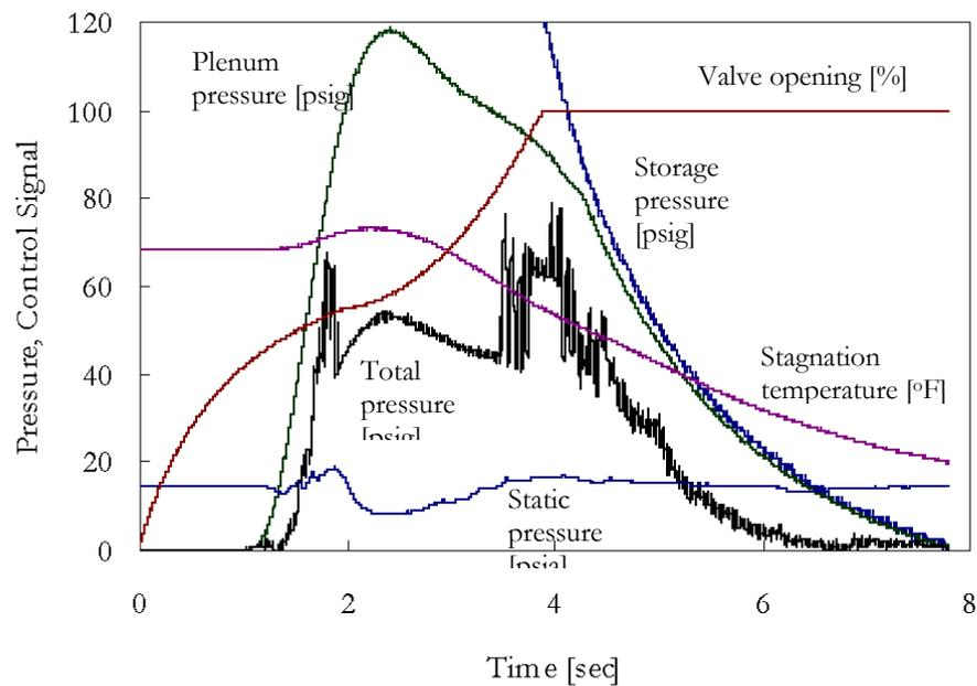
Figure 4.3. Pressure trace of a test with scavenger scoop.
