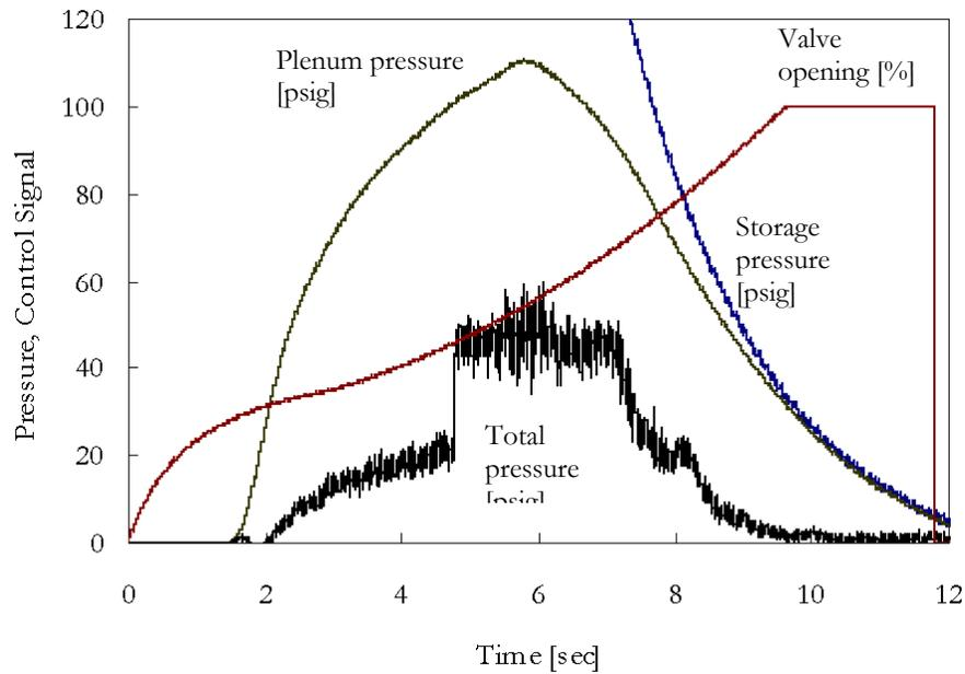
Figure 4.1. Pressure trace of a shakedown test.
