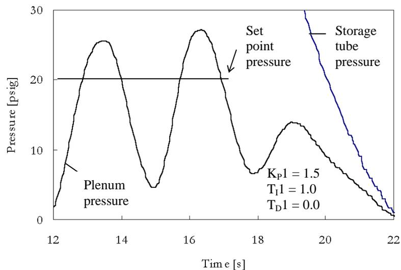
Figure 3.3. Typical plenum pressure trace using PID controller.
