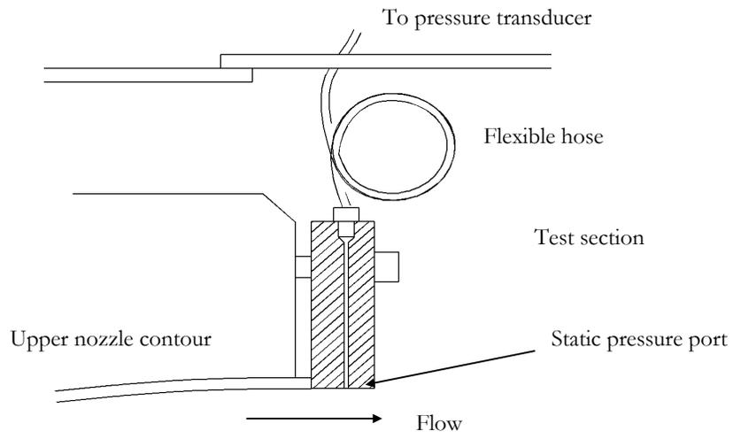
Figure 2.16. Static pressure port.
