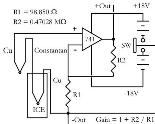
Figure 2.15. Circuit diagram of thermocouple and amplifier.
