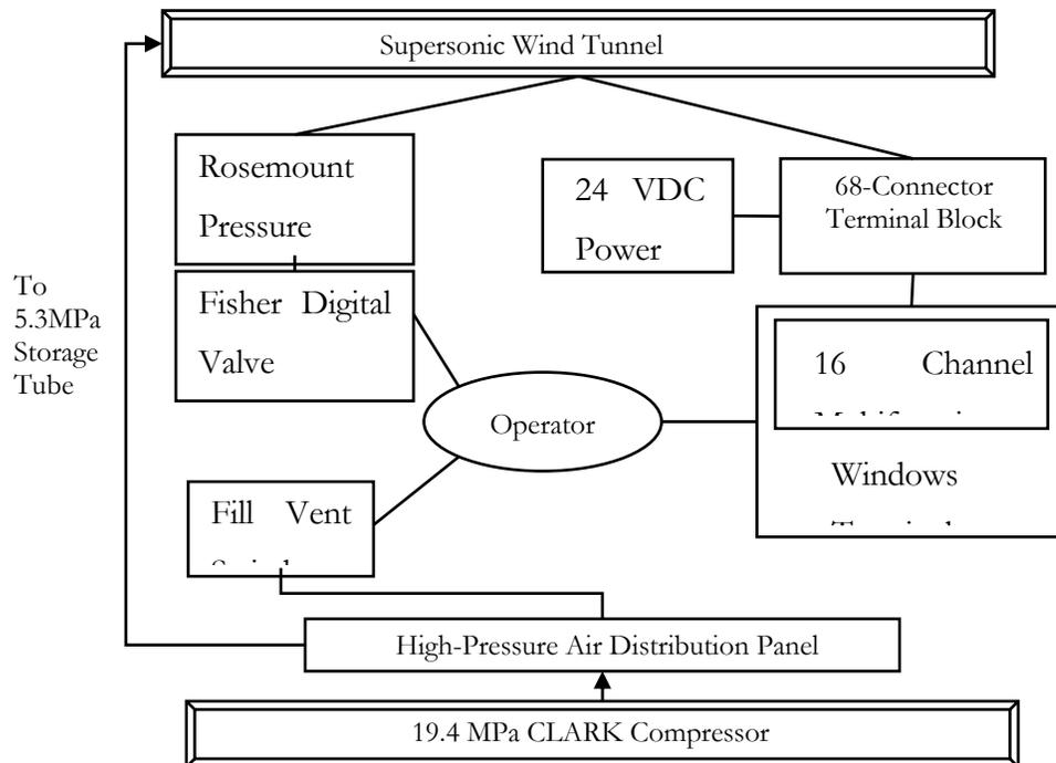
Figure 2.14. Block diagram of tunnel operating system.
