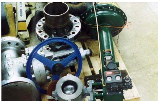
Figure 2.5. Gate valve and automatic valve.
