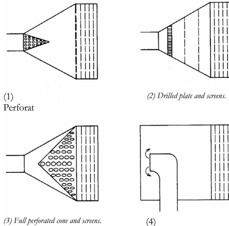
Figure 2.6. Design of wide-angle diffuser. (1) Perforated can plus perforated plate and screens. (2) Drilled plate and screens. (3) Full perforated cone and screens. (4) Reverse entry and screens.
