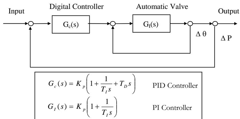
Figure 3.2. PID controller block diagram.
