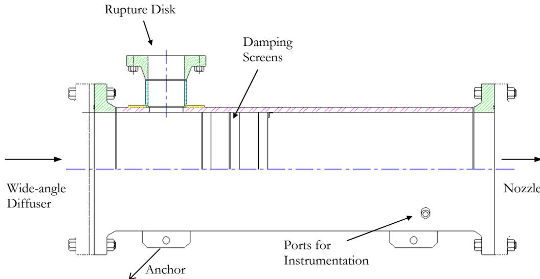
Figure 2.8. Schematic of plenum chamber.
