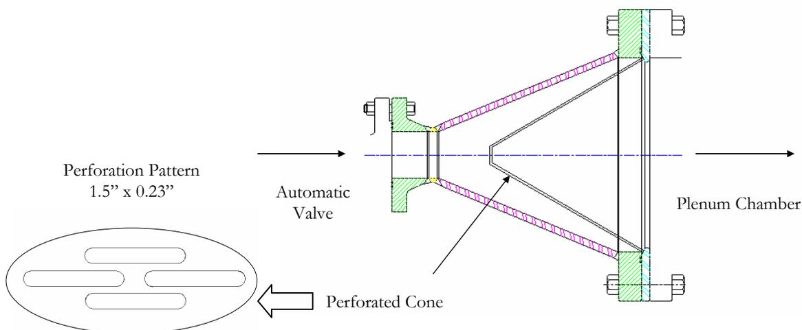
Figure 2.7. Schematic of wide-angle diffuser.
