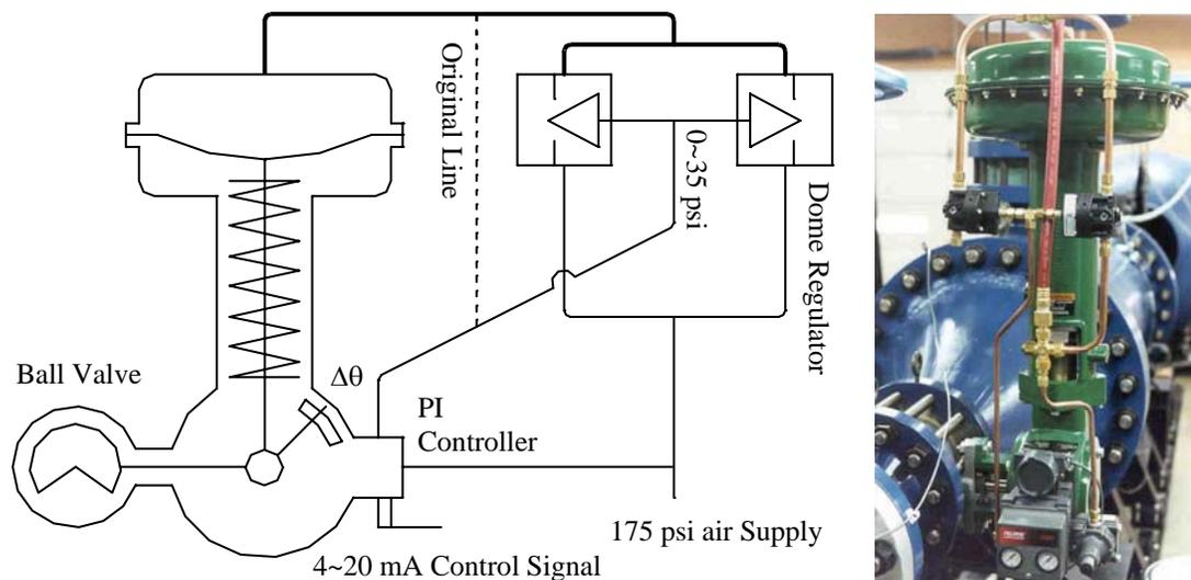
Figure 3.4. Modified pneumatic line of automatic valve.
