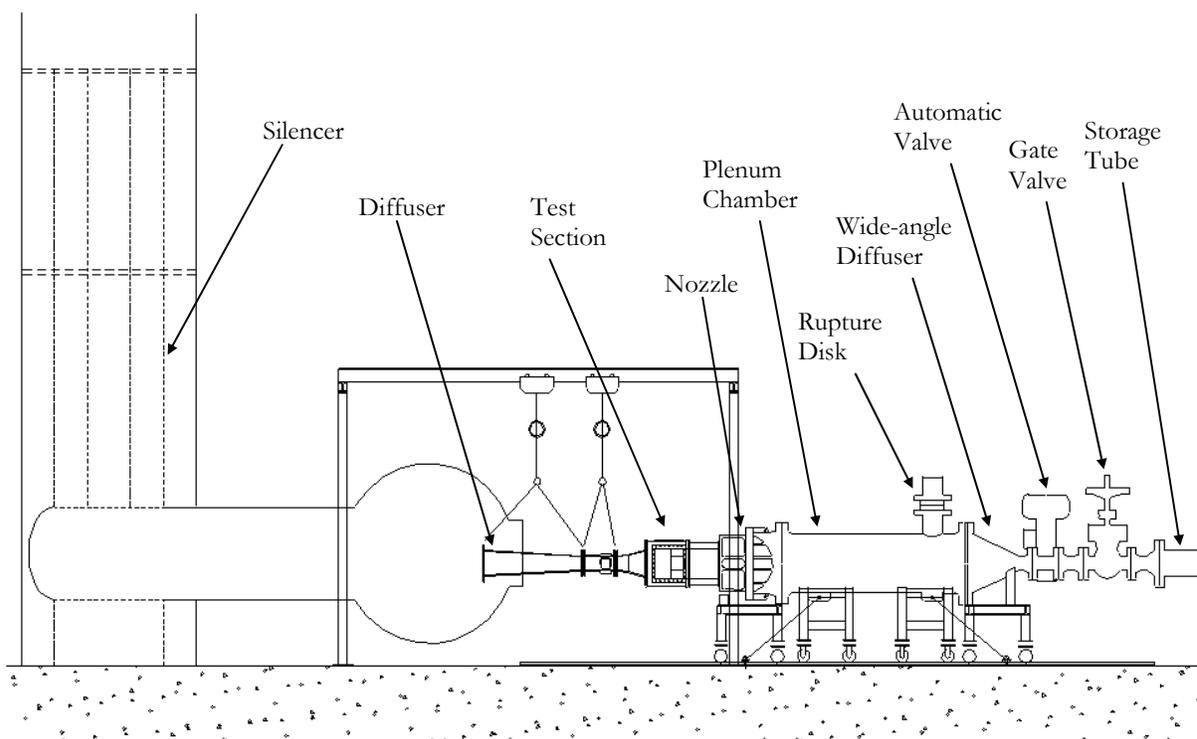
Figure 2.4. Schematic of supersonic wind tunnel.
