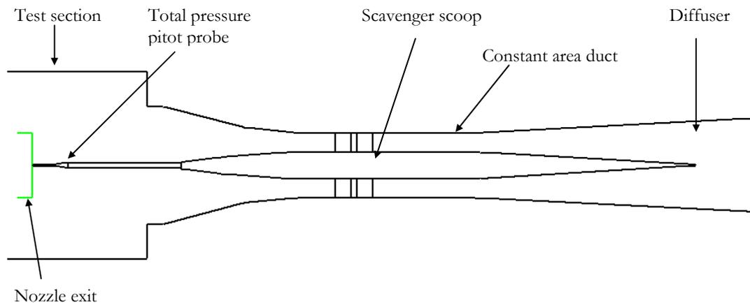
Figure 2.13. Schematic of scavenger scoop.
