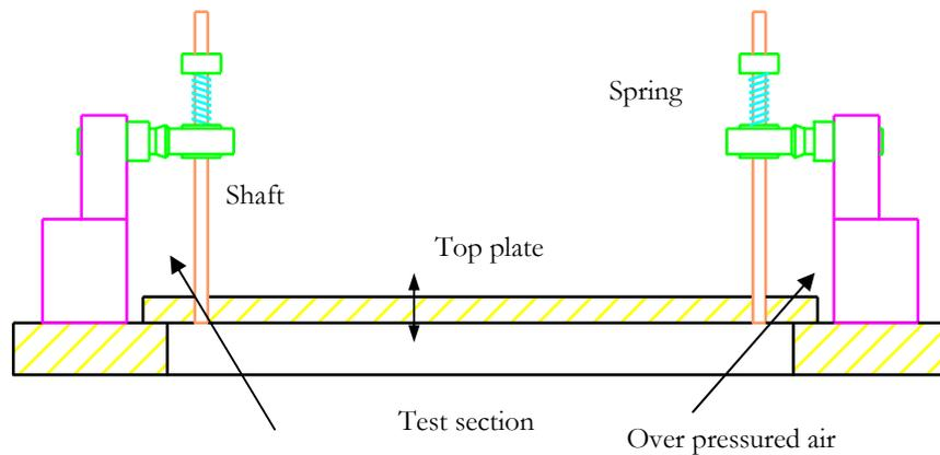
Figure 4.2. Pressure relief plate.
