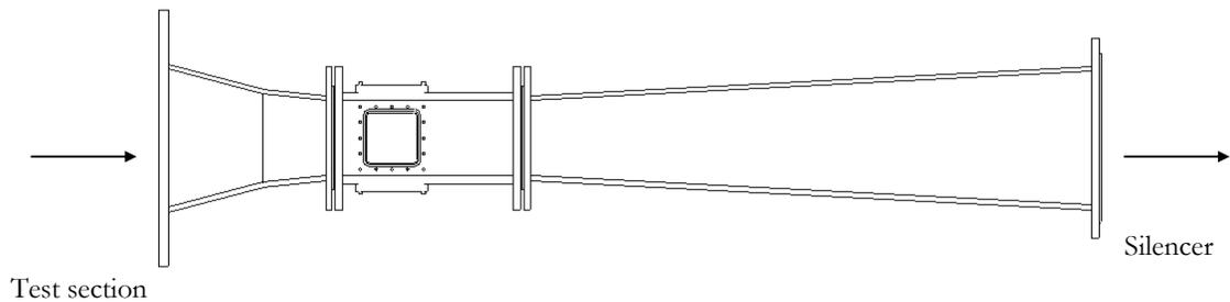
Figure 2.12. Schematic of diffuser.
