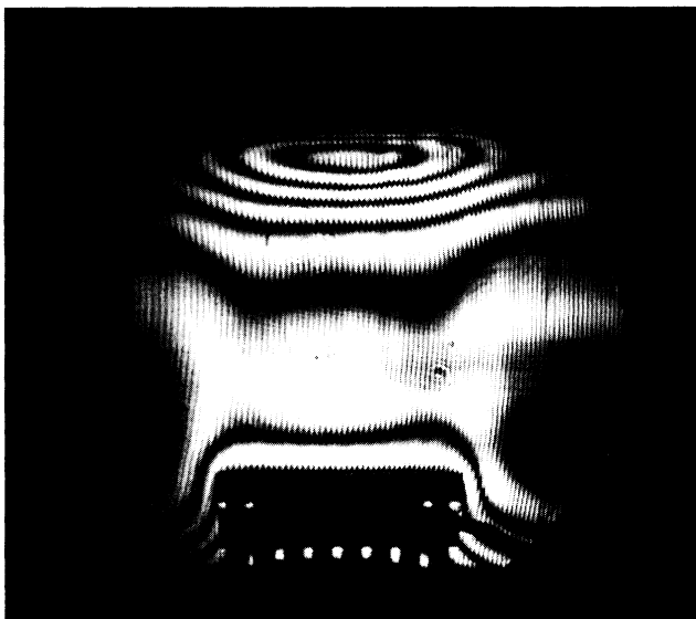
Fig. 7 Interferogram corresponding to heat-flux visualization. The object is an electronic chip mounted longitudinally. The temperature of the chip surface is 225°C as measured by a thermocouple.
