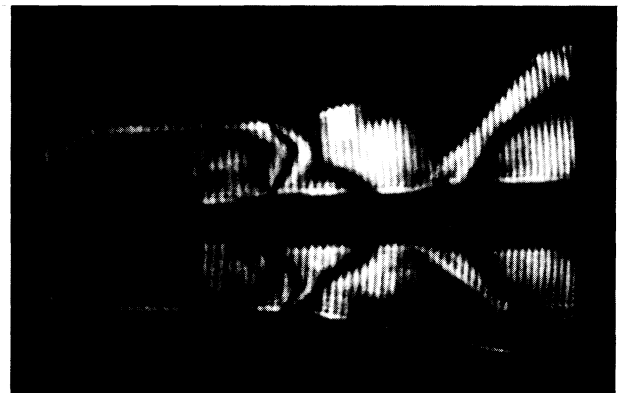
Fig. 2 Interferogram produced by the reconstruction of two double-exposure holograms. The aerodynamic test object is a cylinder with a hole on the tip and an extended slit along its side. The diameter increases gradually in two regions. The vertical fine-line pattern is due to multiple internal reflections in the crystal.
