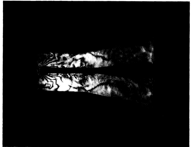
Fig. 14 IR-enhanced recording of flow field inside the window test area. The object is a circularly symmetric rod with a ball tip.
