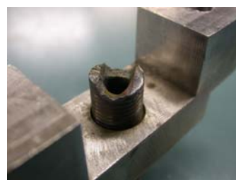
Fig. 1 Erosion of a high-energy arc ignition plug.
