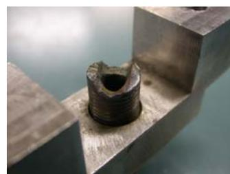
Fig. 1 Erosion of a high-energy arc ignition plug.
