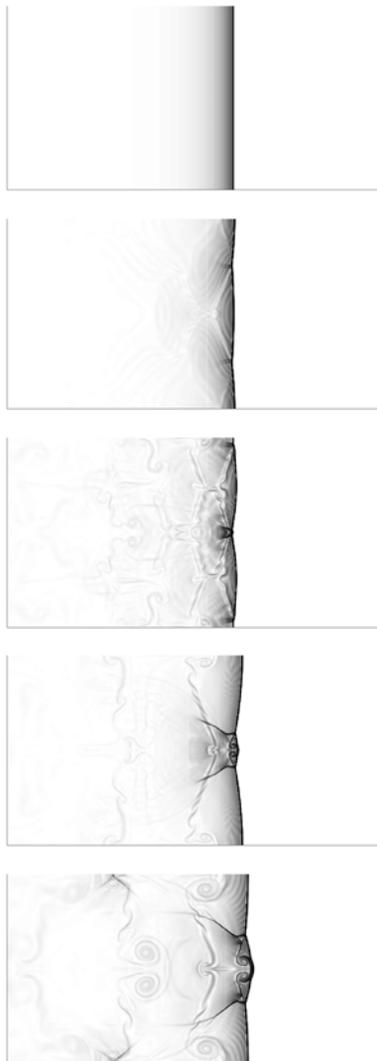
**Fig. 3** Density-gradient plots of a propagating detonation wave
