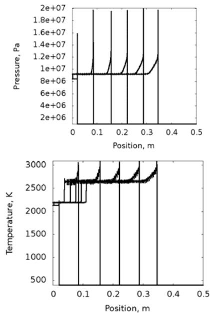
**Fig. 4** One dimensional pressure and temperature profiles of a propagating detonation wave
