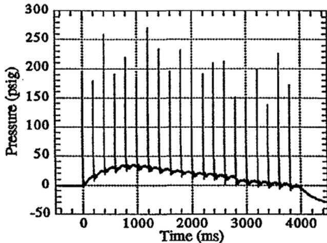
Figure 11. Example showing thermal drift of piezo-electric transducer output [61].
