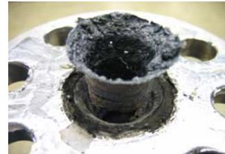
b. The remainder of the spiral that has melted and fused together.
