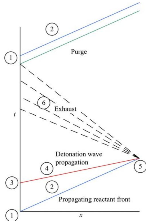
Figure 3. PDE unit process.
