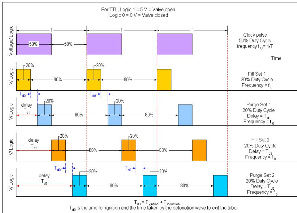
Figure 6. A schematic of the TTL control signals for injection valve timing for two sets of valves.
