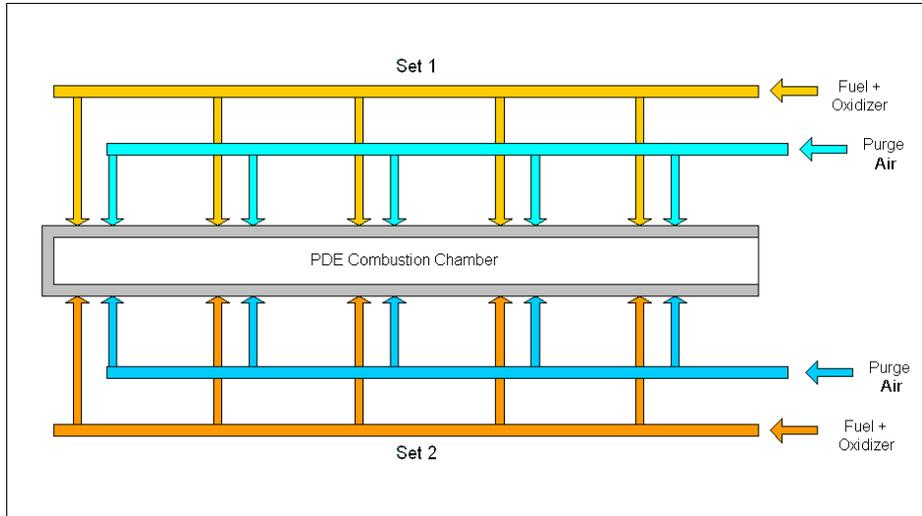
Figure 5. Schematic showing arrays of sidewall injection ports for premix fuel/oxidizer and purge air.
