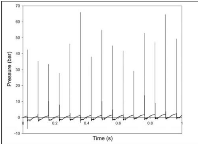
Figure 10. The fluctuation in peak pressure due to low sampling rate.
