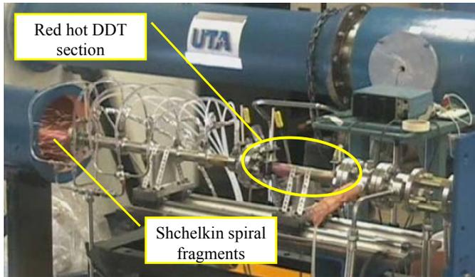
**Figure 7. A PDE without cooling showing red hot DDT section after a few seconds of testing.**
