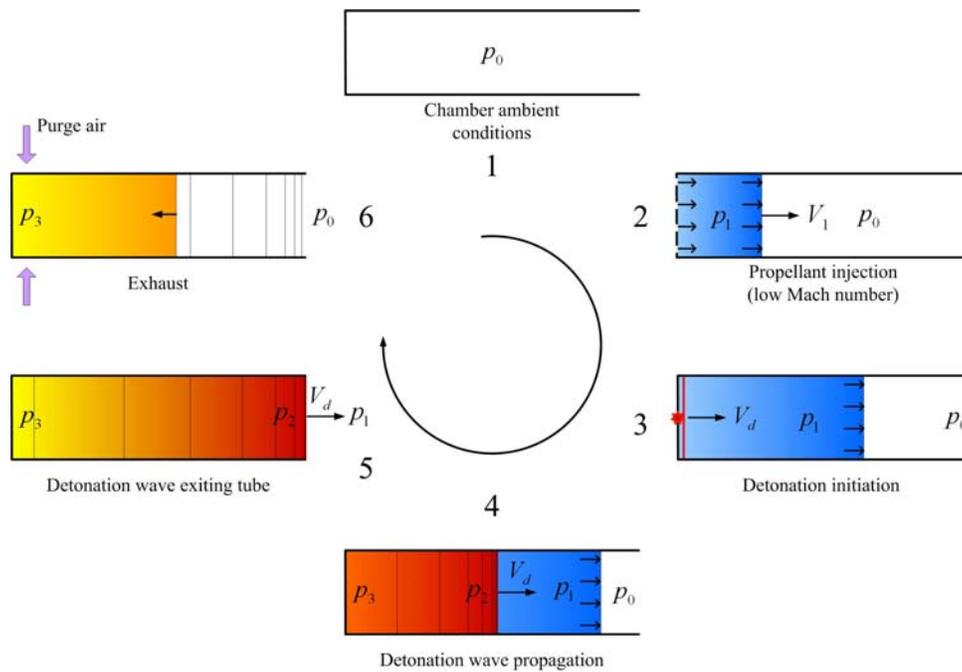
Figure 2. Stages of a PDE cycle.
