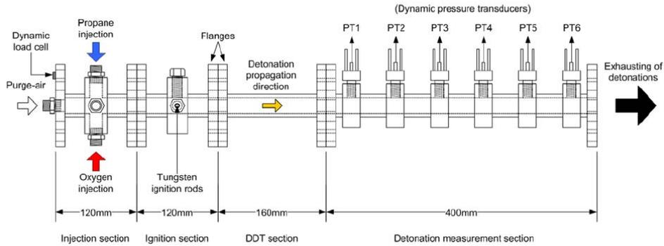
Figure 1. Schematic of a PDE operating with propane and oxygen [15].
