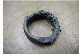
a. A broken piece of the spiral recovered from the PDE tube.
