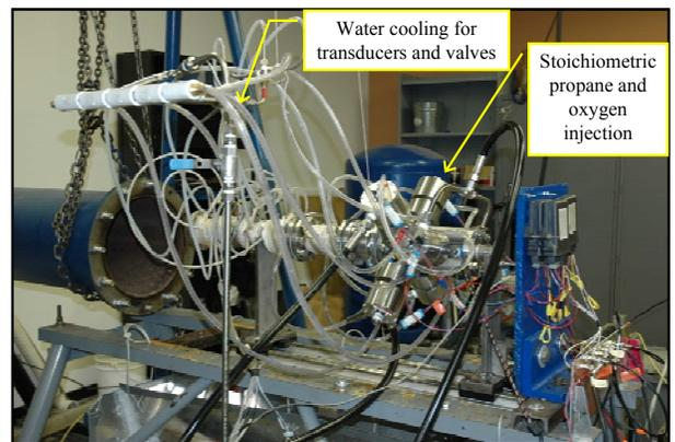
**Figure 9. A water-cooled PDE.**
