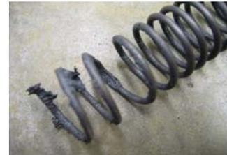
c. Parts of the spiral have been compressed and parts of it has melted away leaving residue.
