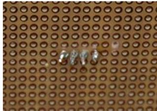
**Figure 7. Four electrodes mounted on a PCB**
