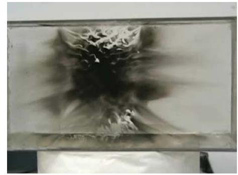
**Figure 16. Sooting on surface of plexiglass top after flame suppression experiment (expanded metal network removed)**
