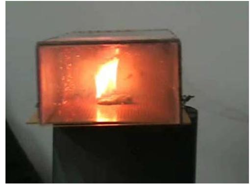
**Figure 15. Successful flame suppression with four layers of expanded metal network in plexiglas container**
