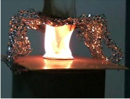
**Figure 13. Successful flame suppression with four layers of expanded metal network**
