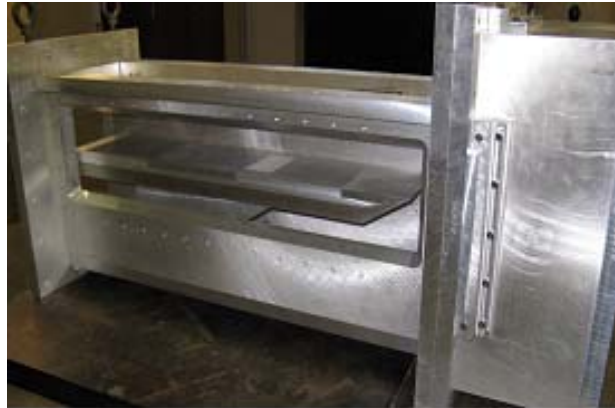
Figure 2. Test section showing flat plate. Flow from right to left.
