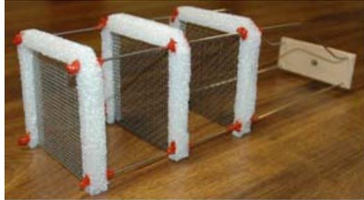
Figure 3. Photograph of turbulence generator.
