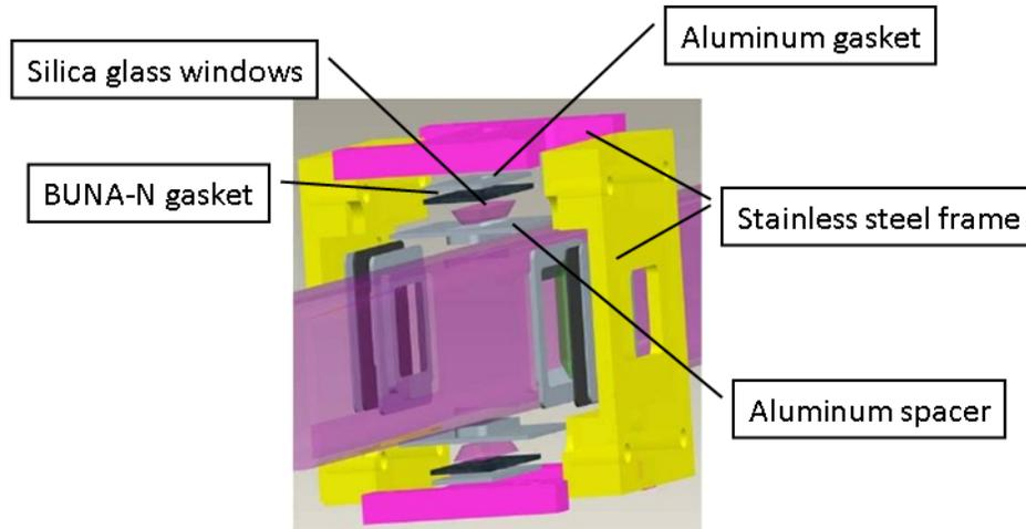
Figure 2. Exploded view of test section.
