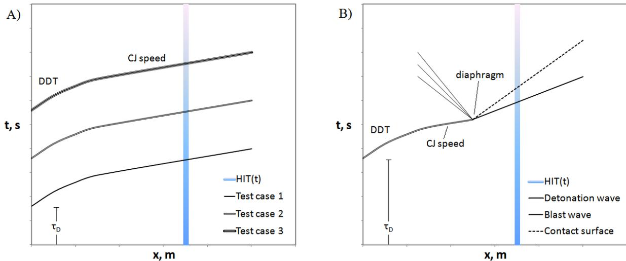
Figure 4. Schematics of time-distance plots for the facility. In A) the grid is moved back to produce the decaying HIT where the ignition delay time  $\tau_D$  in the driver tube is adjusted so the wave interacts with it at different decay points. In B) a diaphragm is used either at the inlet or between driver and driven sections to produce interaction with a shock or blast wave.
