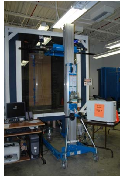
Fig. 4. The Lift Genie for vertically traversing the pair of cameras.
