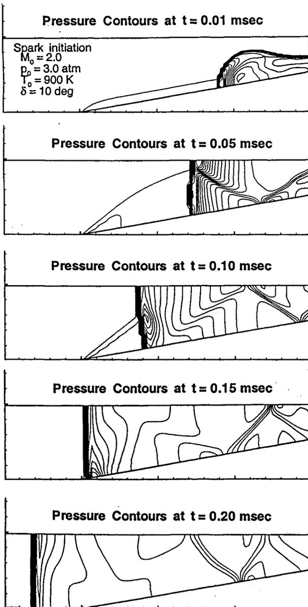
Fig. 5 Upstream propagation of arc-initiated detonation wave on a  $10^\circ$  ramp
