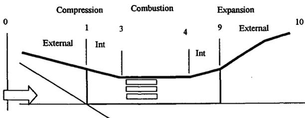
Fig. 10 Engine schematic for stream thrust analysis
