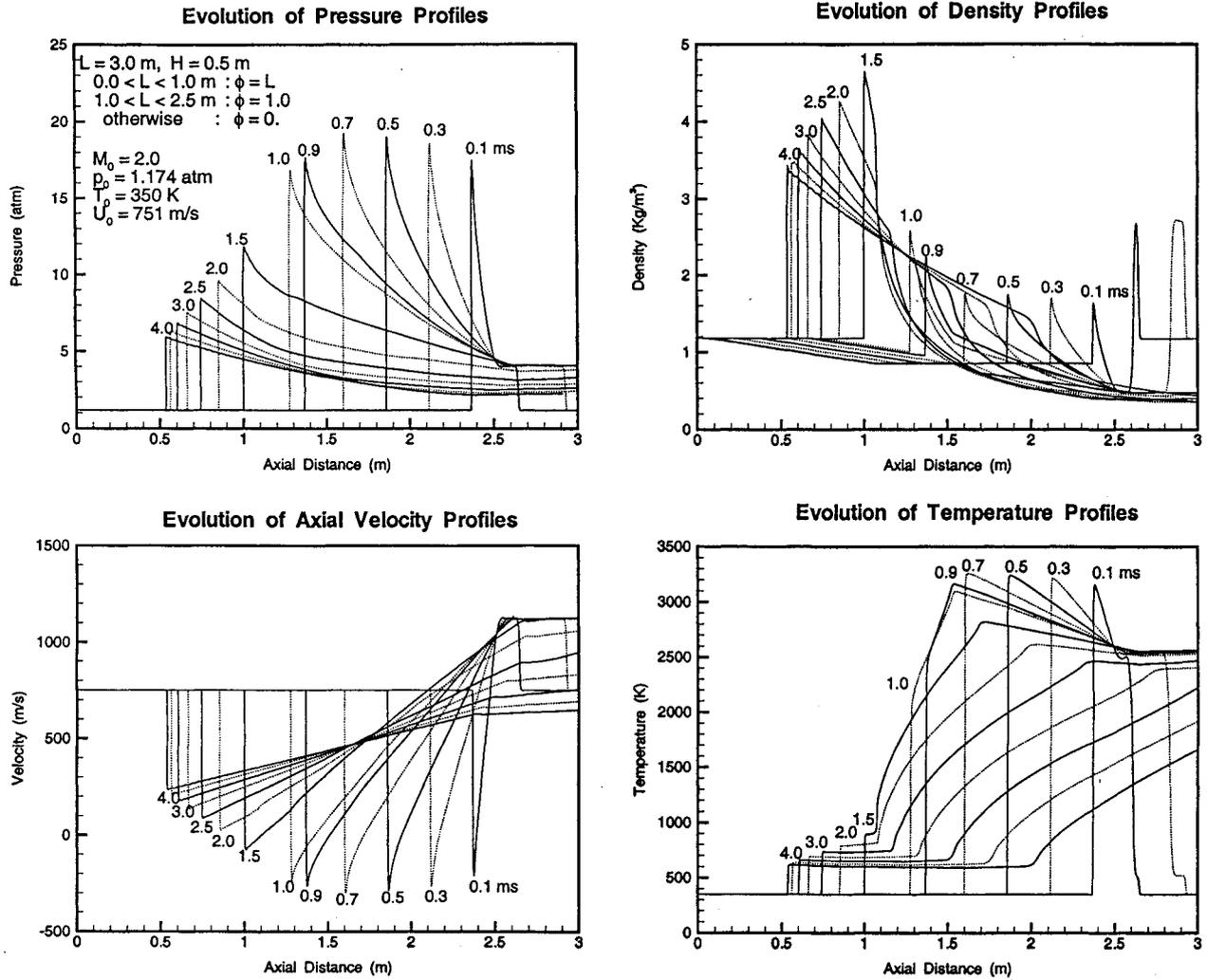
Fig. 9 Pressure, velocity, density and temperature profiles;  $M_3 = 2$ ,  $T_3 = 350 \text{ } ^\circ\text{K}$
