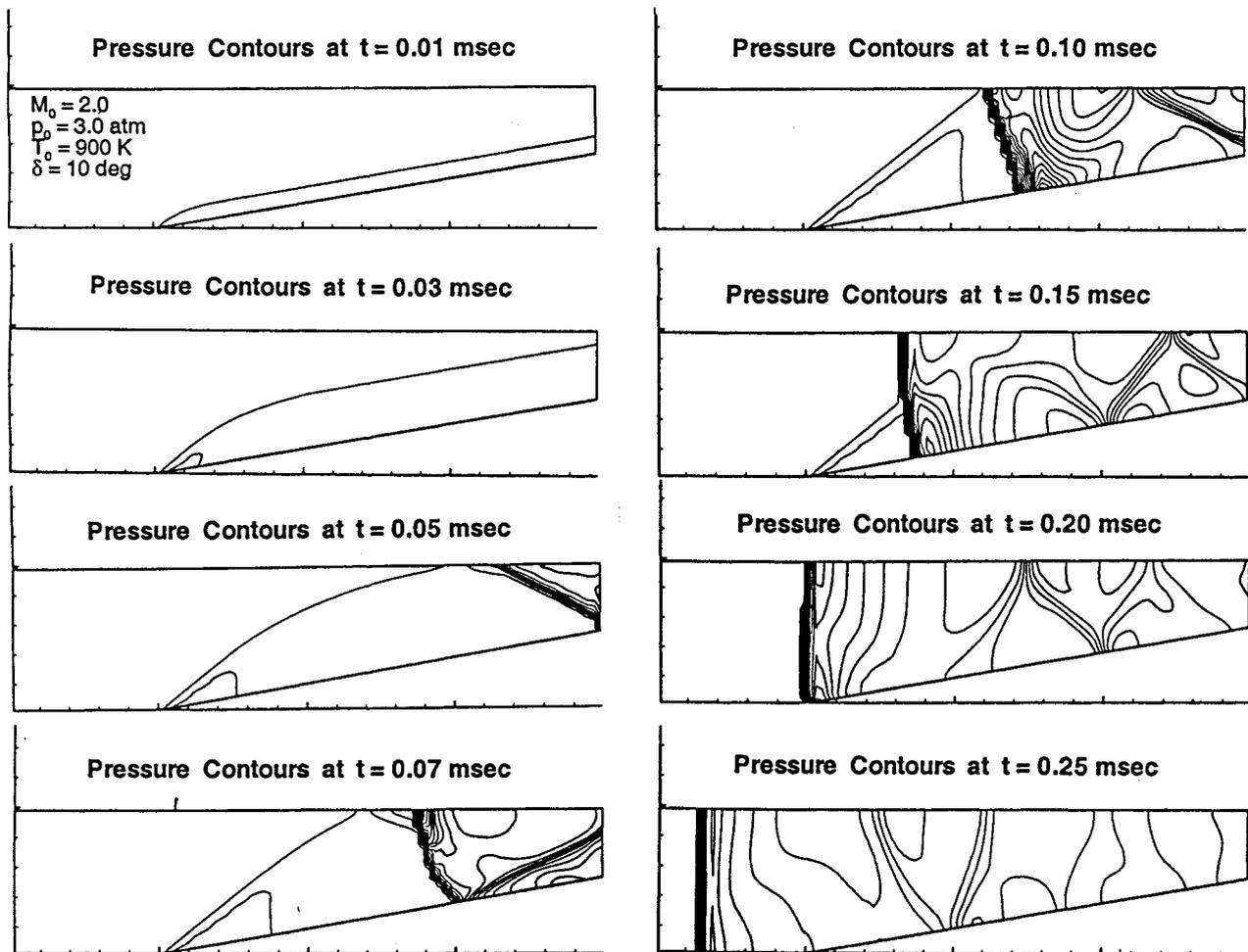
Fig. 6 Upstream propagation of a shock-induced detonation wave
