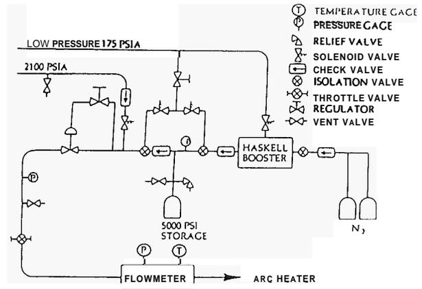
Fig. 9. Schematic diagram - pneumatic system
