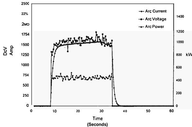
Fig. 14. Arc heater power, current and voltage vs. time
