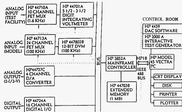
Fig. 10. Schematic diagram - data acquisition system
