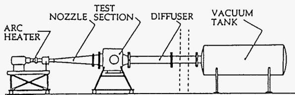
Fig. 2. Elevation view - hypersonic arc tunnel
