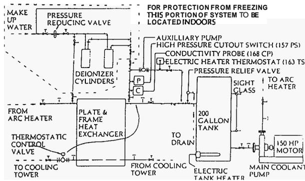
Fig. 8. Schematic diagram - Deionized cooling water system.
