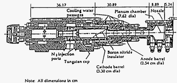
Fig. 4. Cross-sectional view, Thermal Dynamics F-5000 DC electric arc heater
