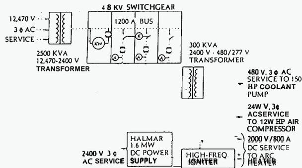
Fig. 6. Schematic diagram - electrical system
