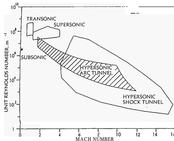
Fig. 1. Aerodynamics Research Center - Experimental simulation capability
