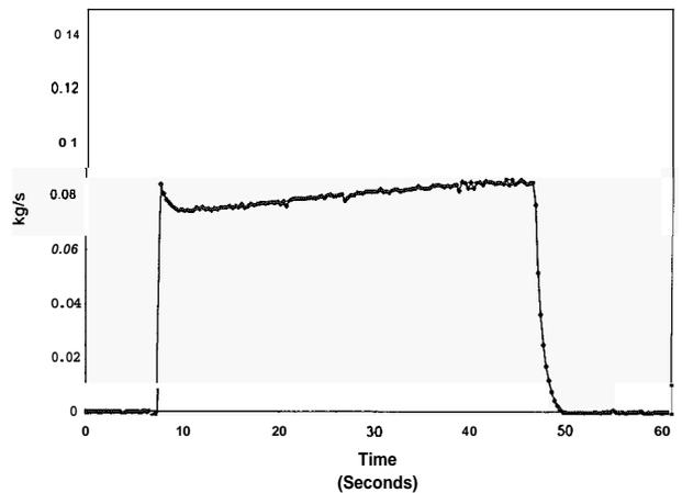
Fig. 16. Nitrogen mass flow rate with unrestricted regulator
