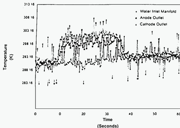
Fig. 12. Typical cooling water temperature-time traces
