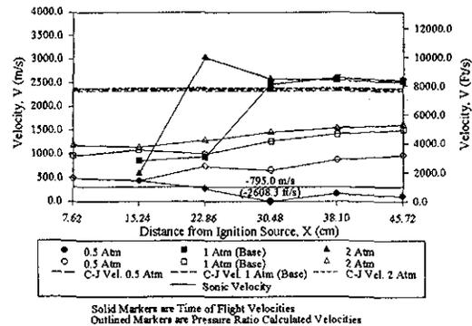
Figure 5.4: Velocity Plot for Propane at Initial Pressures of 0.5, 1 and 2 Atm
