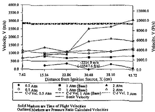
Figure 5.3: Velocity Plot for Hydrogen at Initial Pressures of 0.5, 1 and 2 Atm
