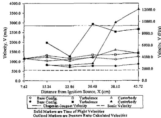
Figure 5.9: Velocity Plot for the Inserts
