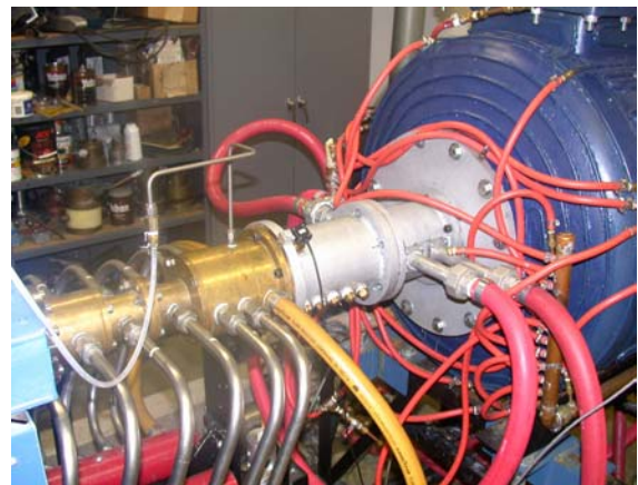
Fig. 7. Photograph of assembled diagnostic chamber.
