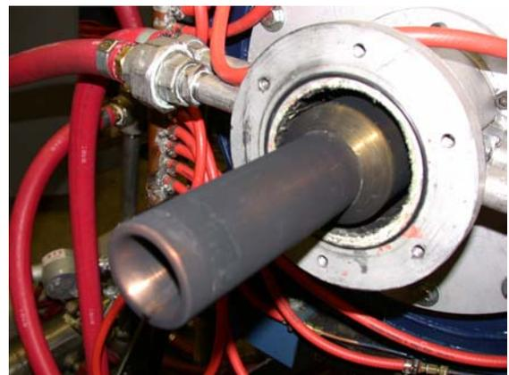
Fig. 8. Carbon deposition resulting from methane pyrolysis.
