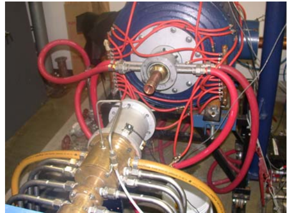
Fig. 6. Photograph of diagnostic chamber showing carbon cold trap.
