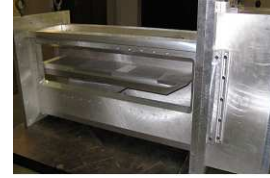
Fig. 3 Test section with side wall removed to show flat plate. Flow from right to left.
