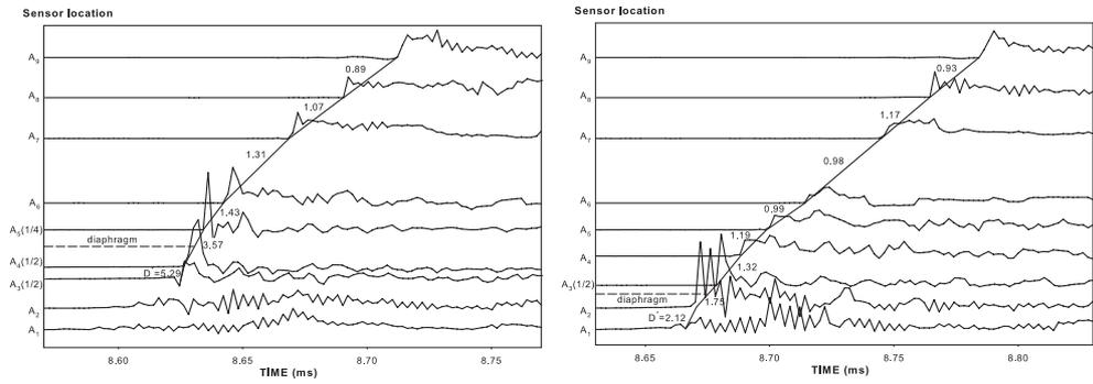
Fig. 4. The displacement-time diagram for mode A1 (left); the displacement-time diagram for mode A2 (right)
