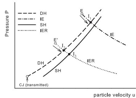
**Fig. 2.**  $P-u$  diagram;  $IE$ : isentropic-expansion curve passing  $D_i$  product;  $IER$ :  $IE$  curve considering rarefaction;  $DH$ : the locus of all possible final states for the  $D_t$ ;  $SH$ : the locus of all possible postshock states
