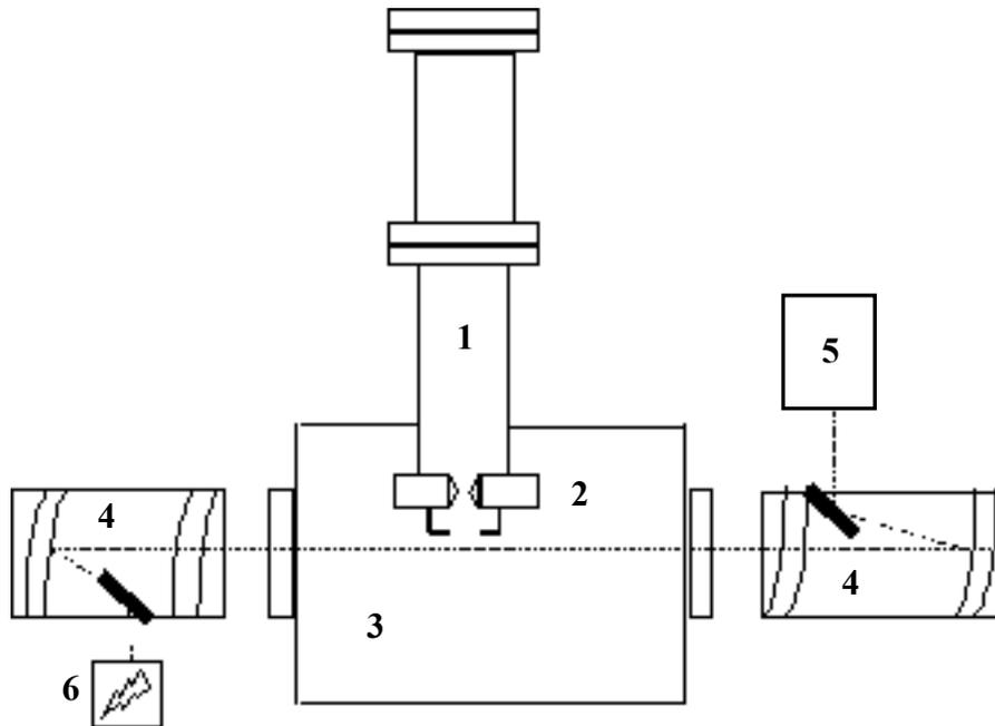
Fig. 1 The experimental setup. 1- shock tube; 2- nozzle; 3- vacuum chamber; 4- shadow device IAB-451; 5- high speed camera VSK-5; 6- light source
