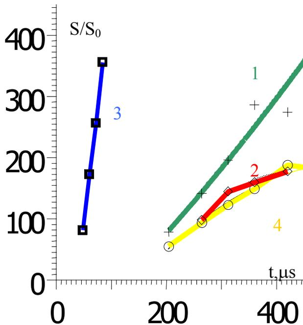
Fig.6 Dependence of the contact surface area of formed jets following from nozzles of the same critical area as function of time; the pressure ratio = 6.6 and mass flux of 33.1 gram/s: curve 1 – from the whistler nozzle (green), curve 2 – from circular supersonic nozzle (red), curve 3 – from sonic generator (blue), the pressure ratio = 4.05 and total mass flux = 21.1 gram/s: curve 4 – from the whistler nozzle (yellow)
