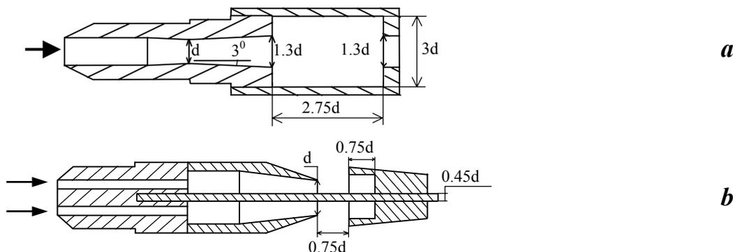
Fig. 2. Whistler nozzle (a) and acoustic driver (b). Dimensions are presented terms of the critical area.
