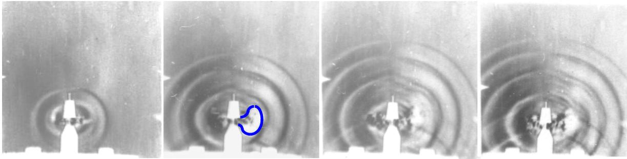
Fig.5 High speed schlieren pictures of sonic generator performance. The ambient pressure is 1 atm, the pressure supply is 6.15 atm. The time moments from the start of the process are 72  $\mu$ s, 156  $\mu$ s, 192 $\mu$ s, 228  $\mu$ s.
