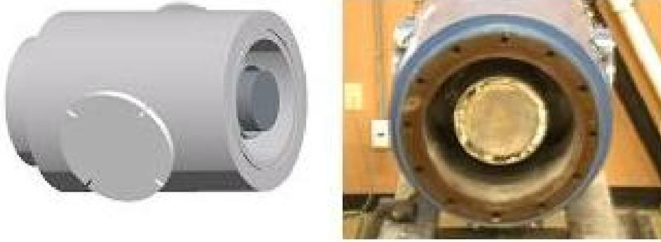
**Fig. 1.** Schematic side view and front view on the concrete cylinder mounted in the test section.
