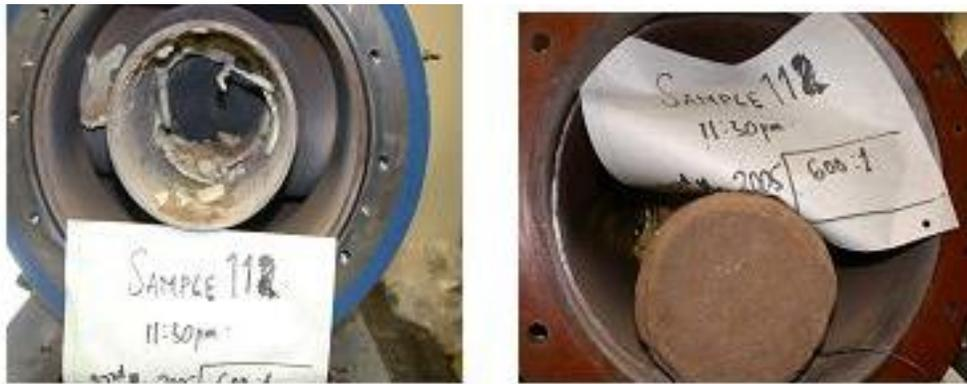
Fig. 3. Cylindrical sample in the nozzle section after testing at  $M = 2.82$ .
